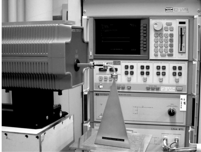
Fig. 2 Photograph of the millimeter wave measurement system
