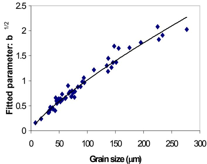
Figure 6. Calibration of the fitted attenuation parameter 'b' and metallographic measured austenitic grain size.
