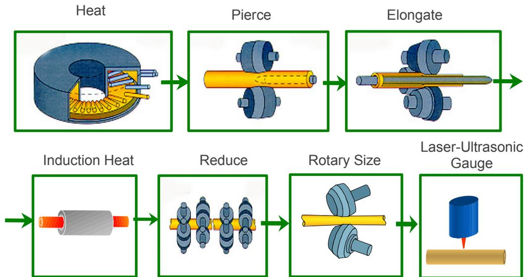
Figure 1. Stages of a seamless tube producing process.
