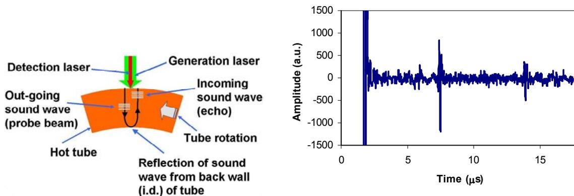
Figure 3. (a) Principle of laser ultrasonic generation and detection in a tube and (b) signal acquired on-line for a 16 mm thick tube at 940 °C.
