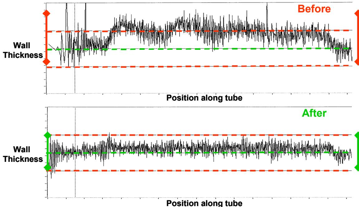
Figure 6. Example of a tube detected within specification only at its very ends and then, after corrective measures, the next tube produced within specification along the entire length.
