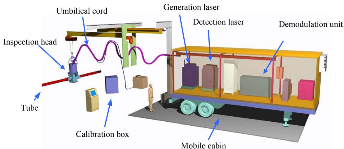
Figure 4. Overview of the laser ultrasonic system.
