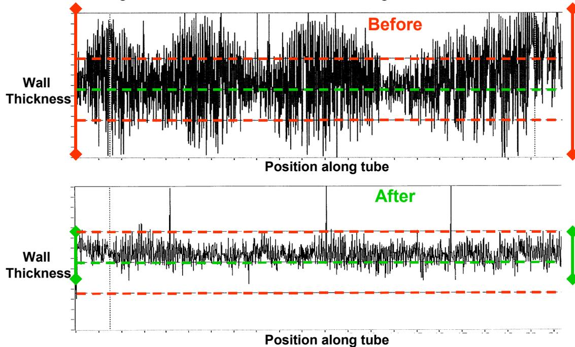
Figure 5. Example of a tube detected with high eccentricity exceeding specification and then, after corrective measures brought to the line, the next tube produced within specification.
