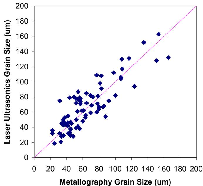
Figure 7. Grain sizes measured on-line by the laser ultrasonic system as a function of those obtained by metallography on the same tubes after proper quenching.
