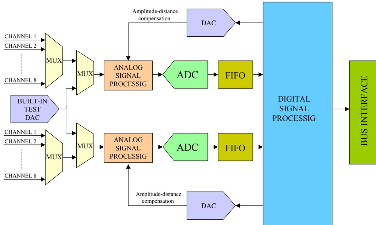
Figure 3. Internal architecture of TU-200 ultrasound processing board
