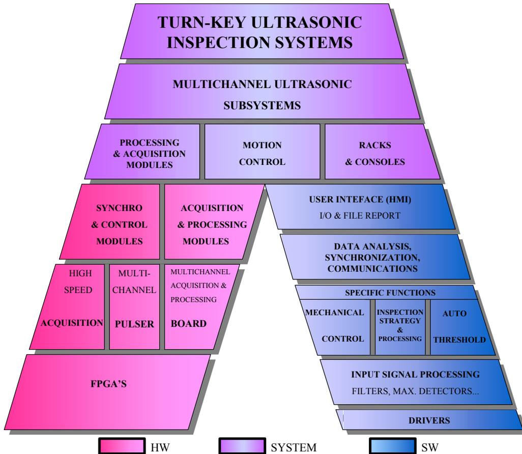
Figure 1. Main components of automatic inspection systems
