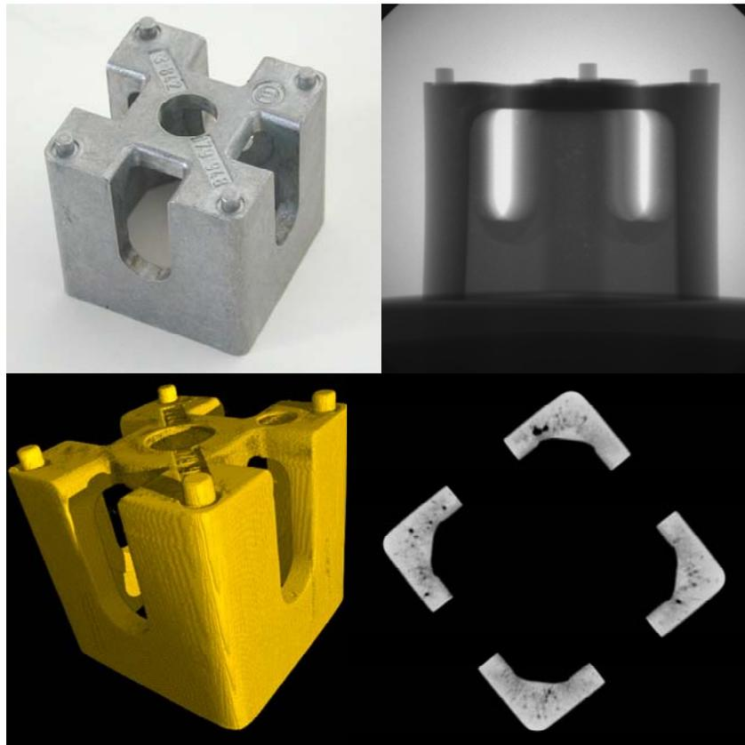
Figure 3: Inside of 3D Micro X-ray CT
