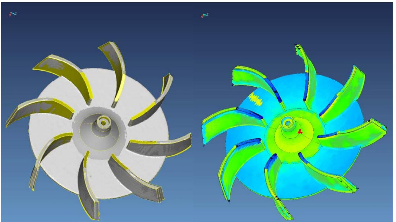
Figure 8: Plastic impeller (l: registered, r: inspection colour plot)
