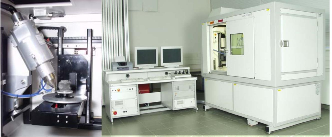
Figure 2: Inside of 3D Micro X-ray CT
