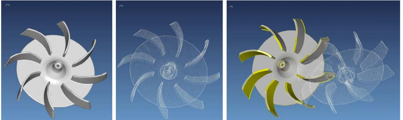
Figure 7: Plastic impeller (l: STL, m: pointcloud, r: unregistered)
