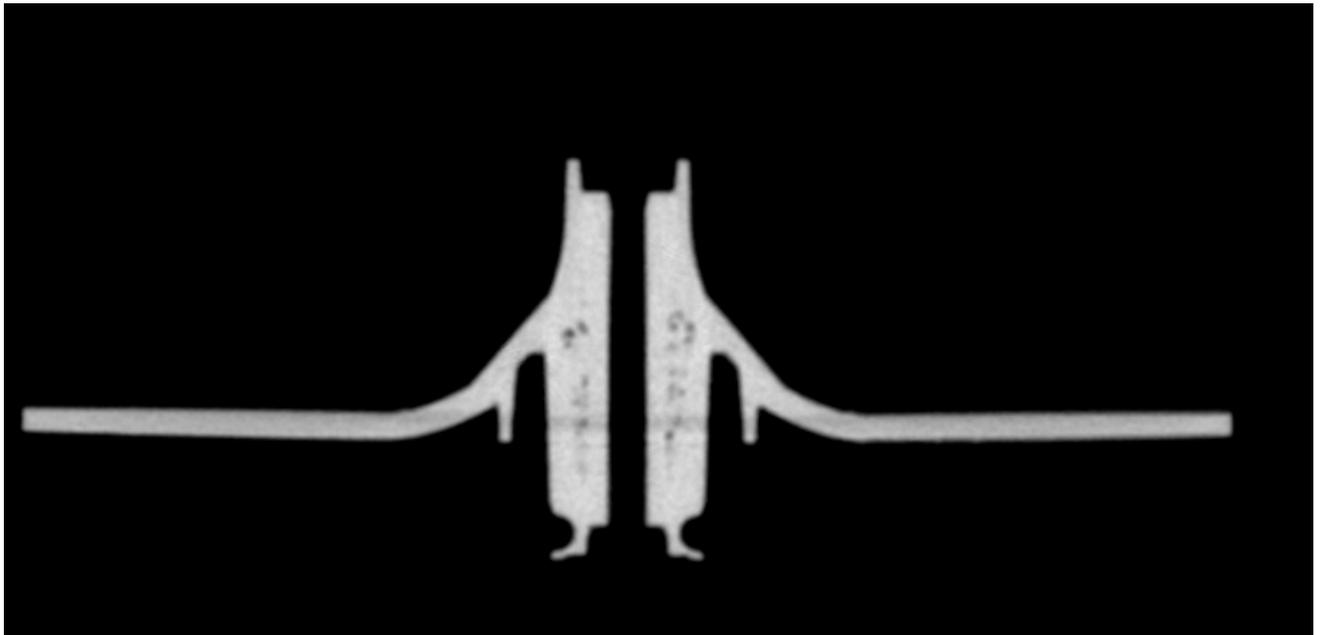
Figure 6: Slice through plastic impeller voxelmodel
