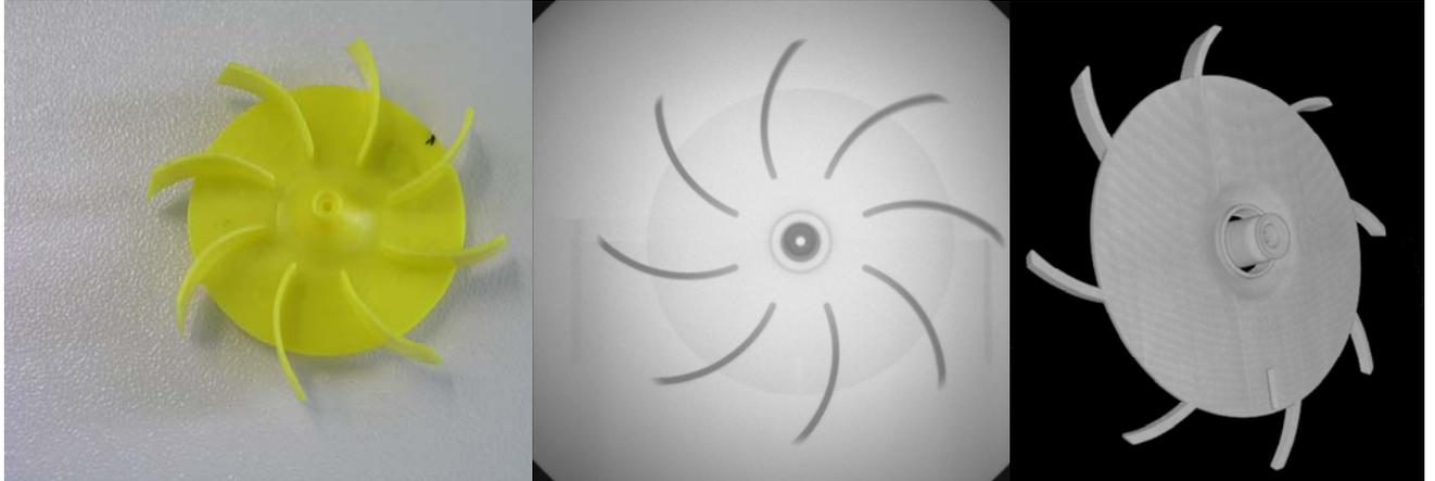
Figure 5: Plastic impeller (l: original part, m: projection image, r: voxel model)
