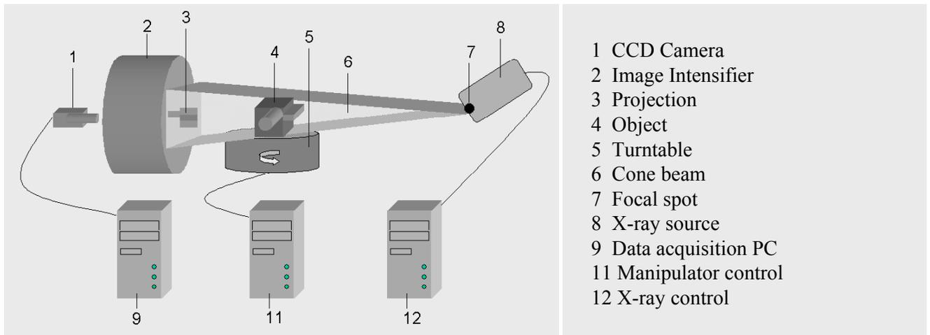
Figure 1: Schematic structure of a 3D CT
