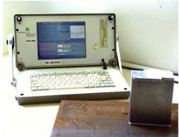
Figure 2: 3MA inspection System
