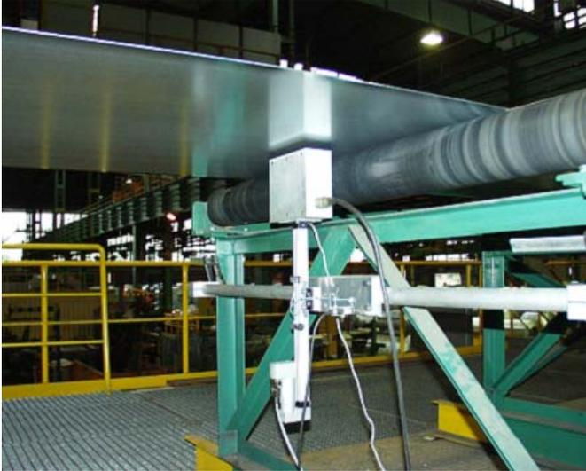
Figure 11: Experimental 3MA installation in a hot-dip galvanizing line
