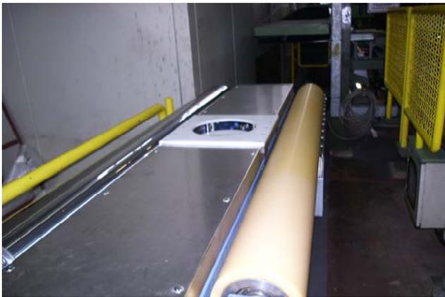
Figure 9: Roller table carrier with integrated transducer
