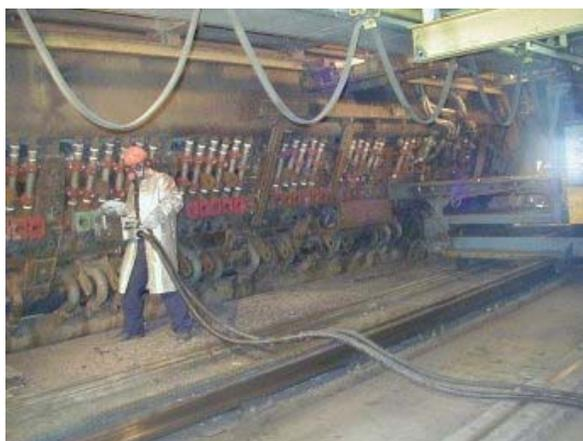
Figure 5. Photograph of the LIBS sensor used on-site for the analysis of molten copper matte
