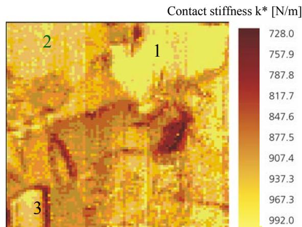
Figure 2: Contact-stiffness AFAM image of Ni
