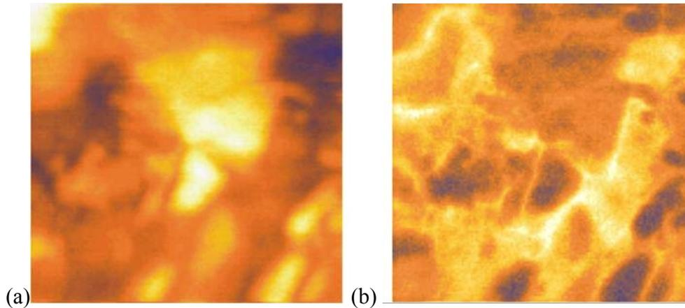
Figure 1: (a) Topography, height scale 10 nm, (b) contact-resonance AFAM image, frequency scale 730 – 750 kHz, of nanocrystalline Ni.
