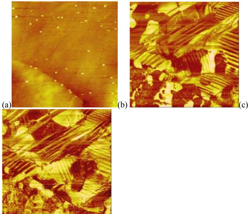
Figure 3: a) Topography, height scale 20 nm, b) vertical and c) lateral piezo-mode images of PIC 1
