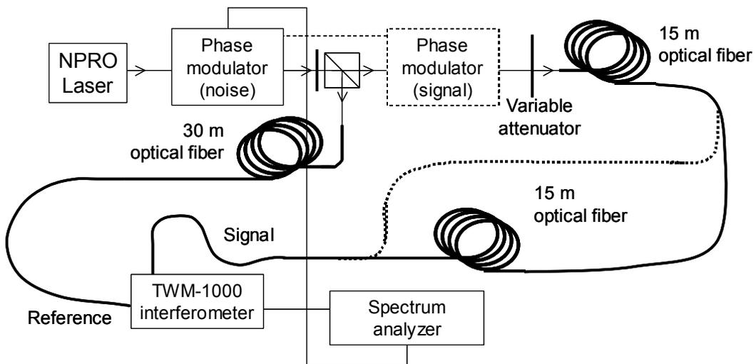
Figure 3 Sketch of the experimental setup to test phase noise rejection by the TWM-1000 interferometer. The phase modulator was positioned either before the beamsplitter (noise position) or after the beamsplitter (signal position). The length of the optical fiber bringing the reference beam to the interferometer had a fixed length of 30 m whereas the total length of the optical fiber bringing the signal beam to the interferometer was either 15 m or 30 m.
