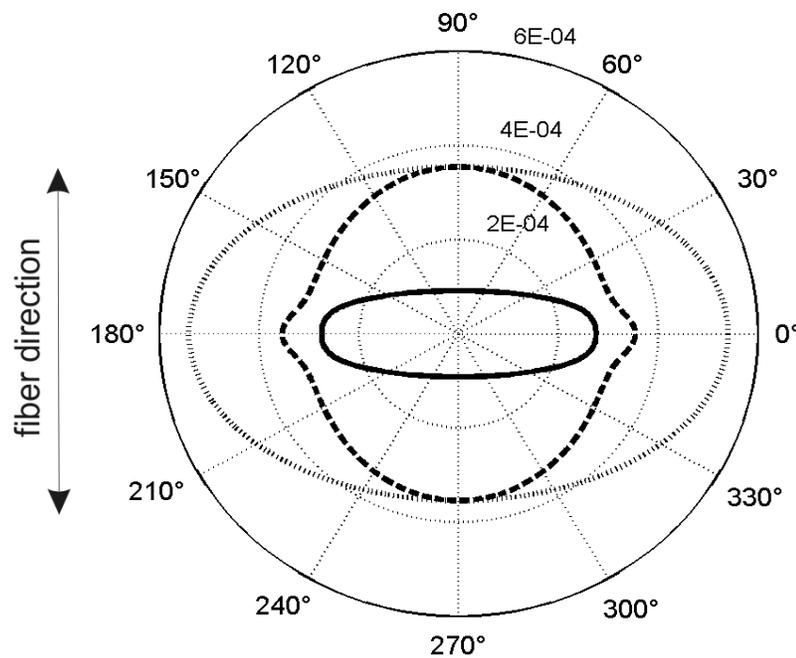
Fig. 4. Section of the slowness surfaces in a plane parallel to the fibers for the MgAl<sub>0,6</sub>/C-M40/70f sample for the longitudinal (solid) and the two transverse waves (dash, dot). The slowness (unit is s/m) is the reciprocal value of the phase velocity.
