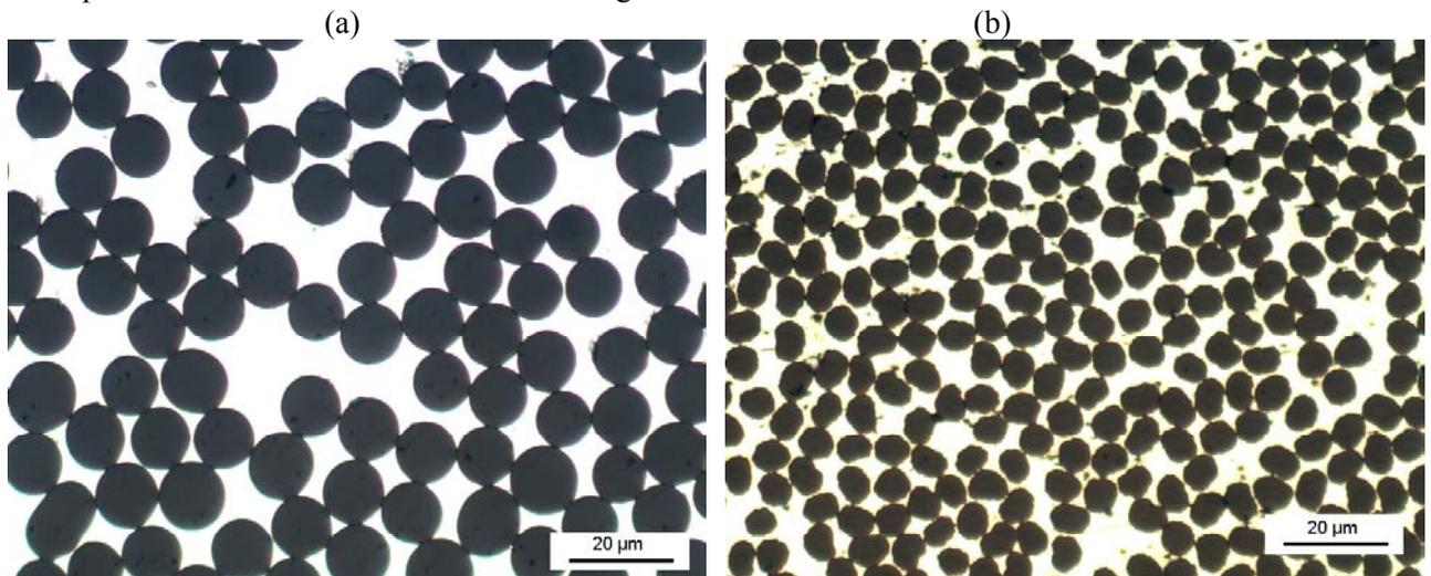
Fig. 3. Lightoptical micrographs of transverse sections of a) AlMg1/Al<sub>2</sub>O<sub>3</sub>-N610/70f, b) MgAl<sub>0,6</sub>/C-M40/70f.
