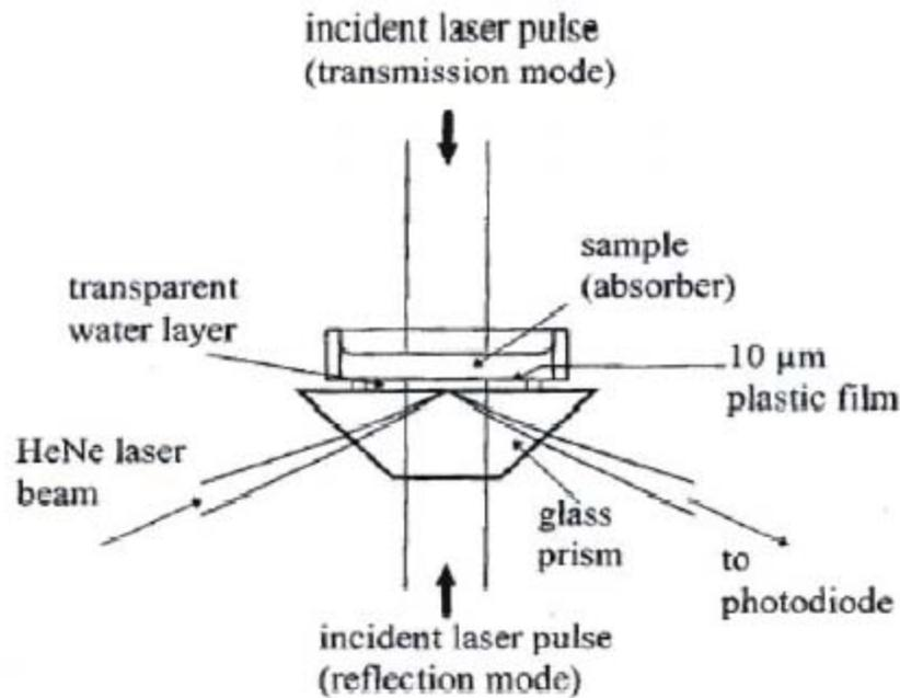
Fig. 1. Laser ultrasound with glass prism as detector [4].
