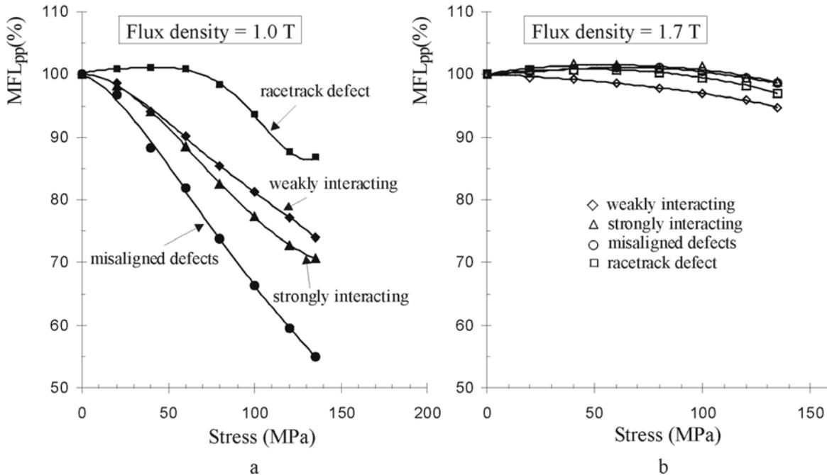
Fig. 3. Radial MFL<sub>pp</sub> percentage change with tensile stress for all defect geometries, in conditions of applied flux densities of (a) 1.0 T and (b) 1.7 T.
