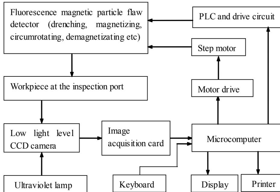
Fig.1 Principle of the fluorescence magnetic particle flaw detecting system
