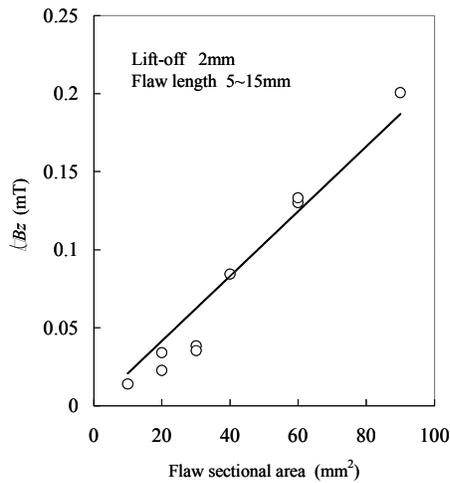
Fig.5 Relationship between  $\Delta B_z$  and sectional area of flaw
