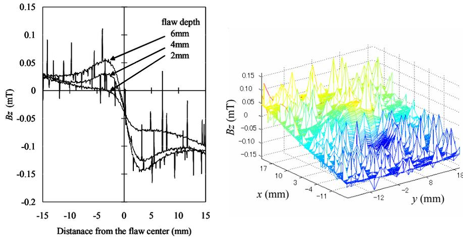
(a)  $B_z$  distributions along the  $x$  axis passing through the center of the flaw (b) Three-dimensional plots of  $B_z$  arising from a flaw of 15mm length and 6mm depth
