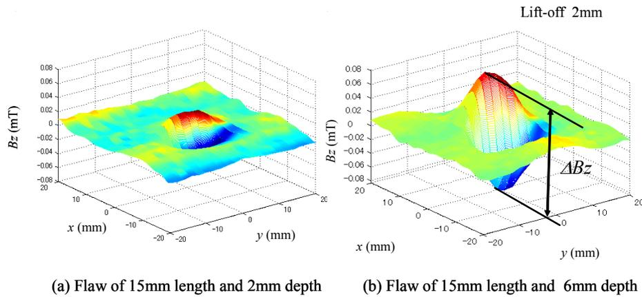
Fig.4 Three-dimensional plots of  $B_z$  after wavelet reconstruction
