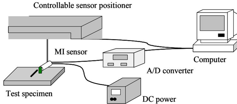
Fig.1 Experimental set-up for residual MFL with MI sensor
