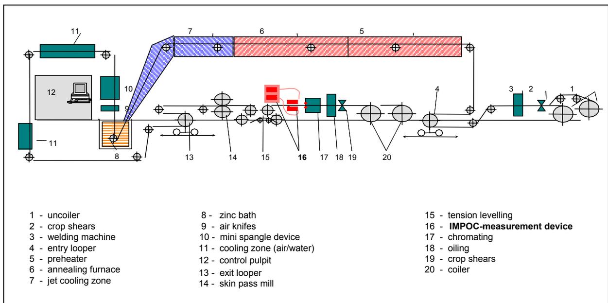
Fig. 3 Layout of the hot dip galvanizing line Nr 1 with IMPOC-1B application
