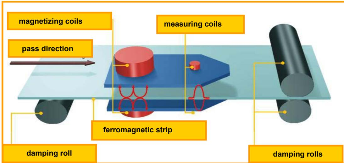
Fig. 2 Structure and measuring arrangement of IMPOC-1B system
