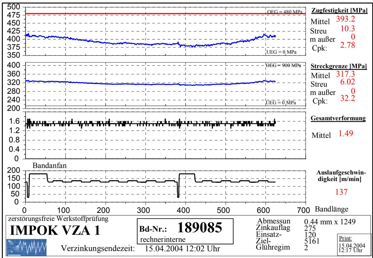
Fig. 4 Quality record of coil Nr. 189085 from the EKO Stahl hot dip galvanizing line 2
