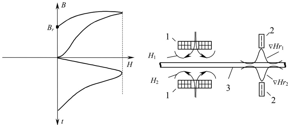
Fig. 1 Measurement principle: 1 – magnetizing solenoids;
