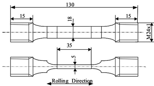
Fig.1 Specimen geometry.
