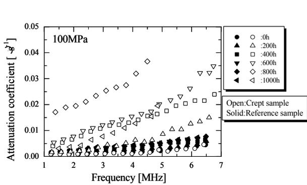
Fig.3 Frequency dependence of the shear-wave for the polarization in the stress direction (Interrupted test, 100MPa, 973K).
