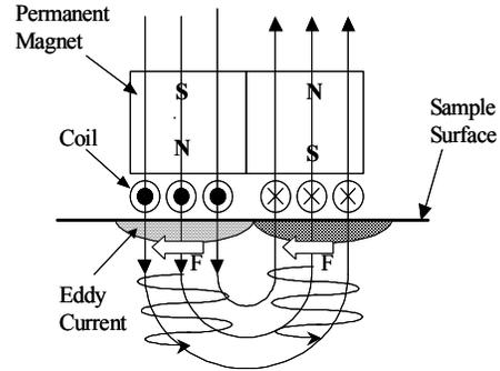
Fig.2 Structure and mechanism of shear-wave EMAT.
