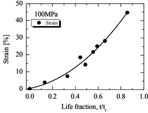
Fig.6 the creep strain reached versus estimated life fraction in Continuous test (100MPa, 973K).
