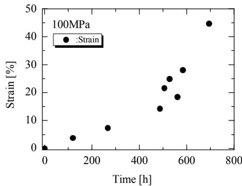
Fig. 5 The creep strains reached versus times in Continuous test (100MPa, 973K).
