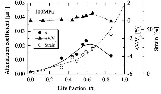
Fig.7 The relationship between  $\alpha$ ,  $\Delta V/V_0$ , creep strain and  $t/t_r$  at the 11th resonant mode under 100MPa in Continuous test (100MPa, 973K).
