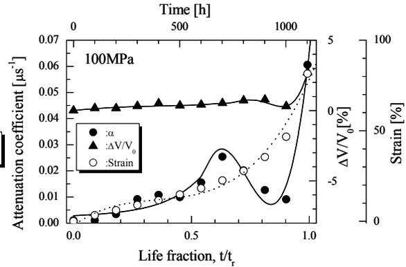
Fig.4 Attenuation and velocity evolutions of attenuation the 11th resonant mode and creep strain. The polarization is parallel to the stress direction (Interrupted test, 100MPa, 973K).
