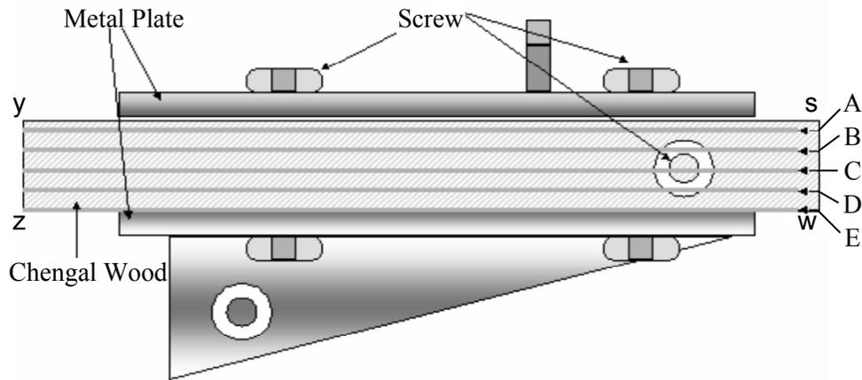
Figure 2 :Experimental Set-Up for Upper method (Top View).
