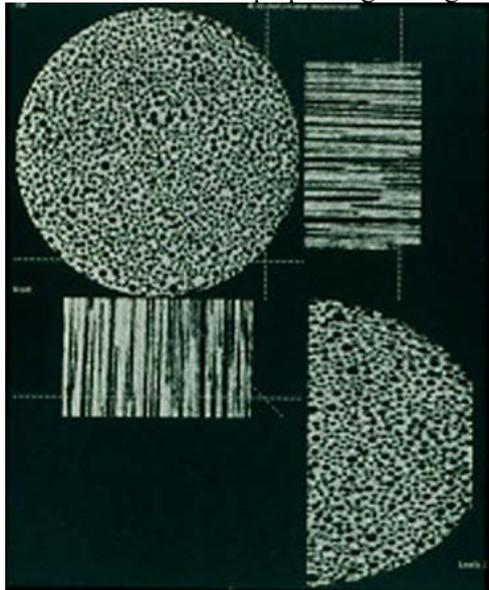
**Figure 3.** Slices of x-ray tomographic images through a metal foam specimen in order to determine if the holes shown on the surface were due to a random distribution of spherical bubbles or tubular in shape passing through the body.
