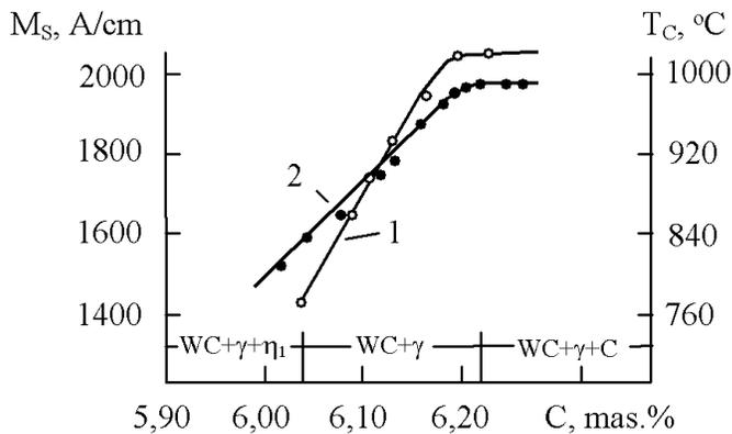
With excess carbon, the isolation of free carbon ( $\text{WC} + \gamma + \text{C}$ ) takes place, whereas with scarce carbon – the isolation of a  $\eta_1$ -phase ( $\text{WC} + \gamma + \eta_1$ ) rich in tungsten and cobalt ( $\text{Co}_3\text{W}_3\text{C}$ ). The isolations of the  $\eta_1$ -phase make the cobalt binder brittle, this being explainable, firstly, by the brittleness of the  $\eta_1$ -phase, and, secondly, by the fact that some cobalt from the composition of the  $\gamma$ -phase
