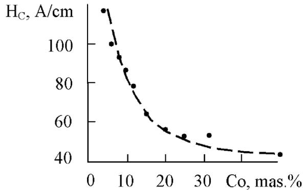
Fig. 4.  $H_C$  as dependent on cobalt content. The dashed curve shows the values of  $H_C$  predicted by eqn (9).  $\langle D \rangle = 3,25 \mu\text{m}$
