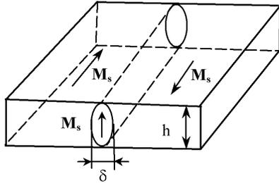
Fig.2. A model of the Bloch wall in a thin magnetic film
