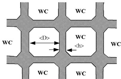
Fig.1. A model of the structure of hard alloys
