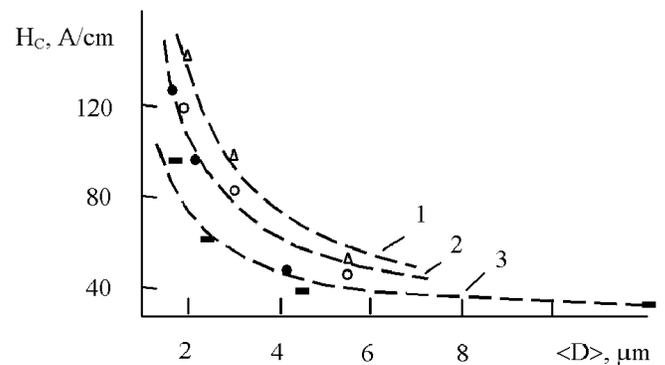
Fig. 5.  $H_C$  as dependent on the mean size of carbide grains for alloys containing: 1 to 8; 2 to 10; 3 to 15 mass percent of Co. The dashed curves show the values of  $H_C$  predicted by eqn (9).
