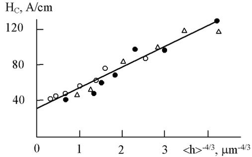
Fig.3. A correlation between  $H_C$  and  $\langle h \rangle^{-4/3}$  for some hard alloy
