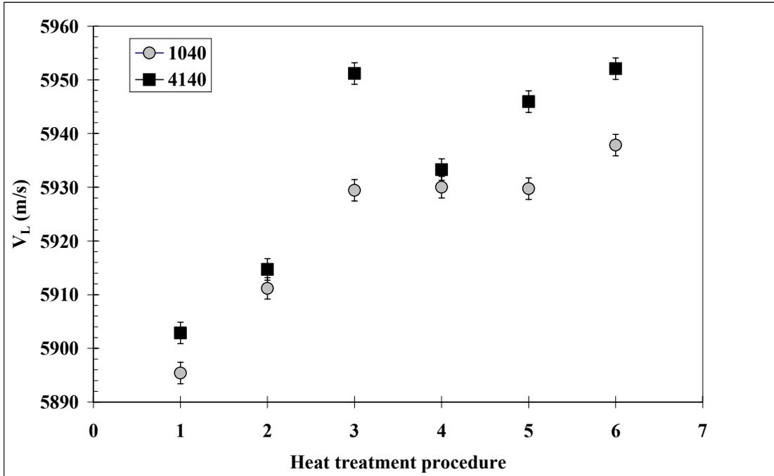
Figure 3. Effect of microstructure on the sound velocity of AISI/SAE 1040 and 4140 steels (1:M, 2:Temp-M 200°C, 3:Temp-M 600°C, 4:Bainite, 5:Fine-P, 6:Coarse-P)
