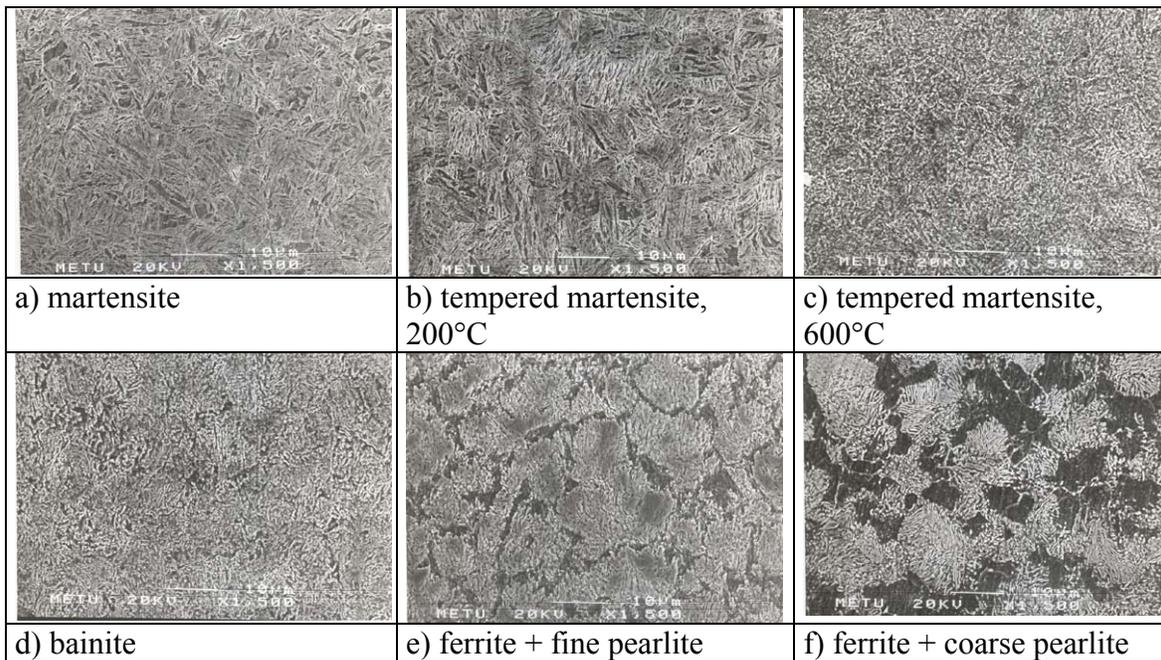
Figure 2. Microstructures of heat treated AISI/SAE 4140 specimens
