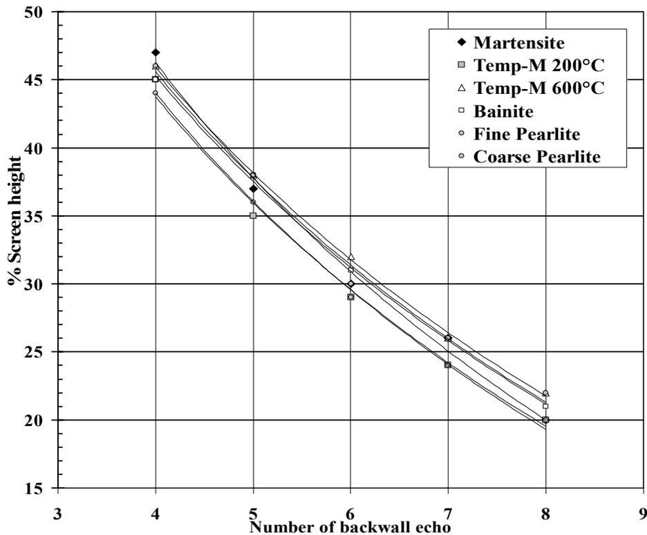
Figure 4. Effect of microstructure on the backwall echo pattern of AISI/SAE 1040 and 4140 steels
