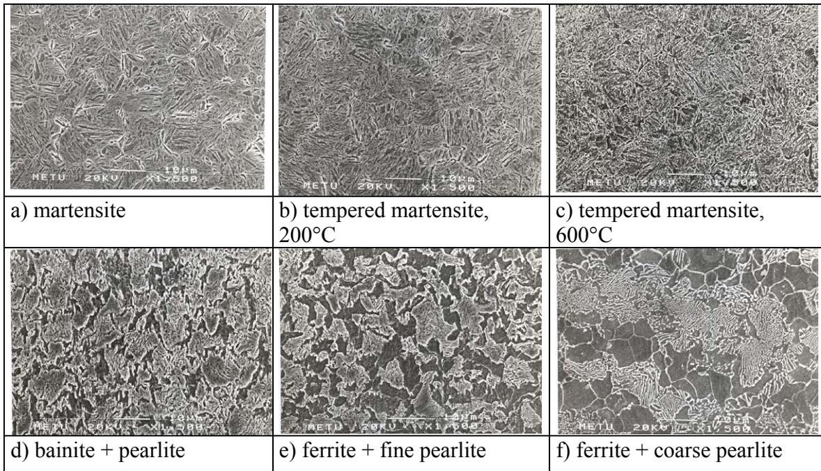
Figure 1. Microstructures of heat treated AISI/SAE 1040 specimens
