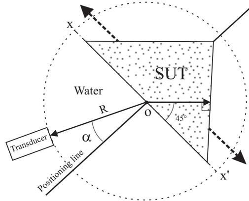
**Figure1: Transducer-cell configuration**
