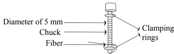
Fig. 3 : Optical fiber rolled on mandrel.
