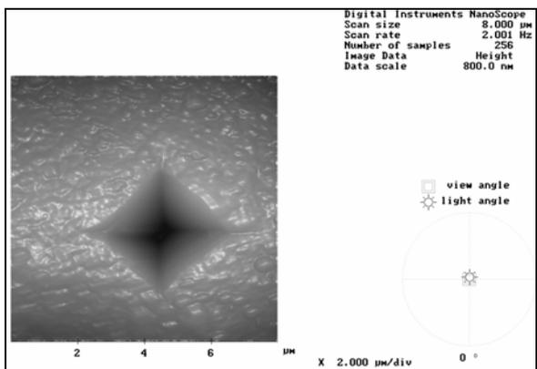
Fig. 8: AFM image of Vickers impression on heat-treated fiber submitted to HF chemical etching.
