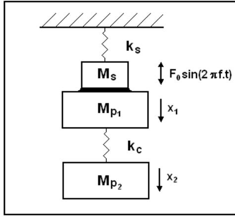
FIGURE 1: Schematically representation of the vibrating system
