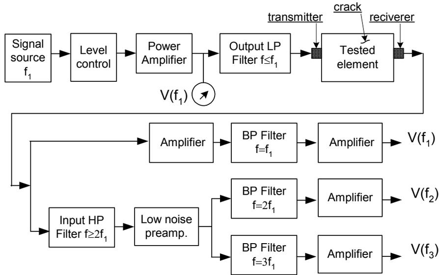
Fig. 3. Block scheme of the measurement equipment
