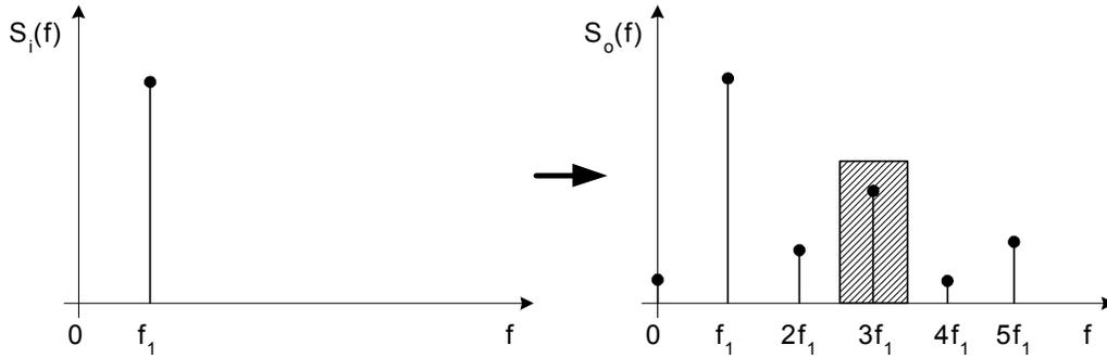
Figure 1.: Growth higher harmonic components in frequency spectra at transit pure harmonic signal through nonlinear environment with illustration of selection dominant third harmonic component by the frequency band-pass filter.
