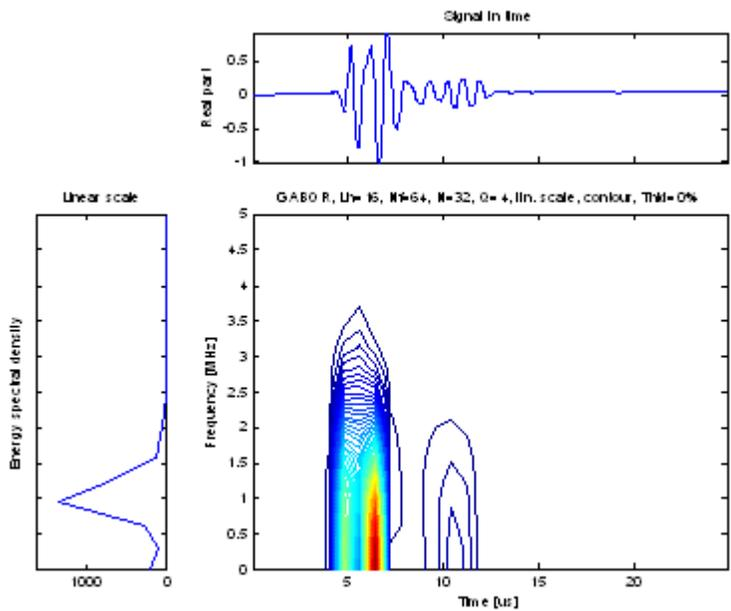
Fig.6 The accurate frequency of ultrasonic pulse echo reflected by flaw
