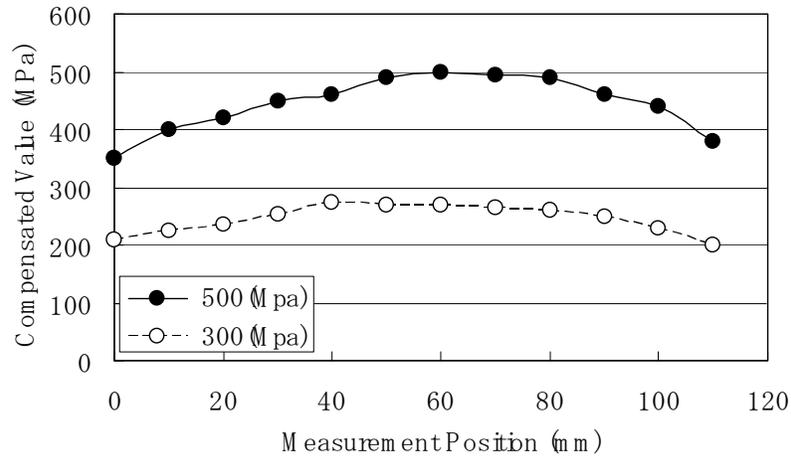
**Fig.8 Stress measurement results along the tensile specimen**
