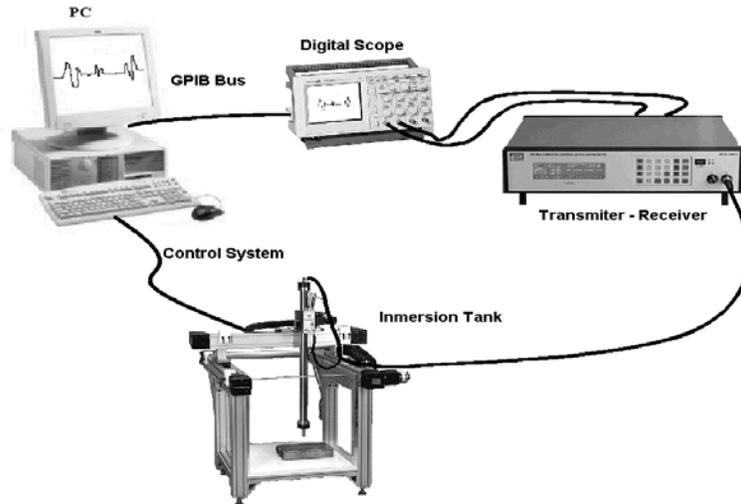
Figure 1.- Experimental set up for the ultrasonic measurements
