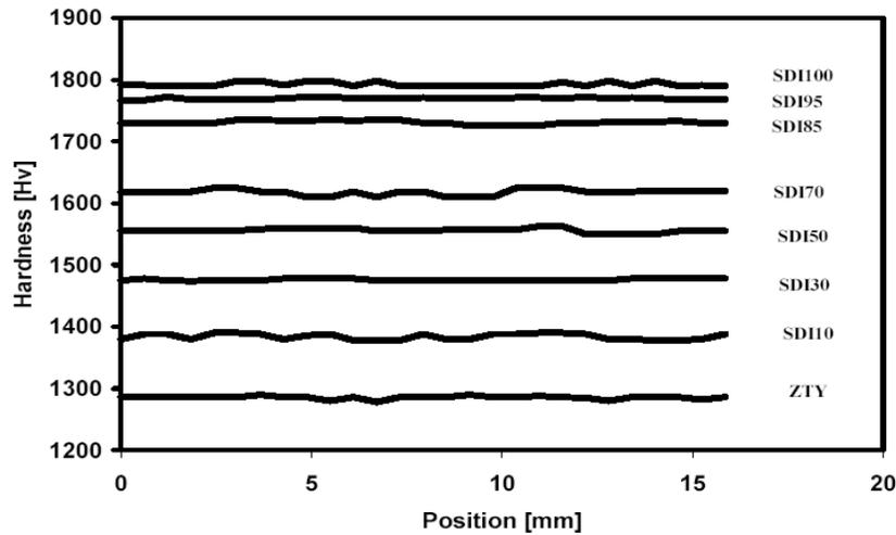
Figure 2.- Vicker's hardness for  $ZrO_2$ - $Y_2O_3$ / $Al_2O_3$  composites
