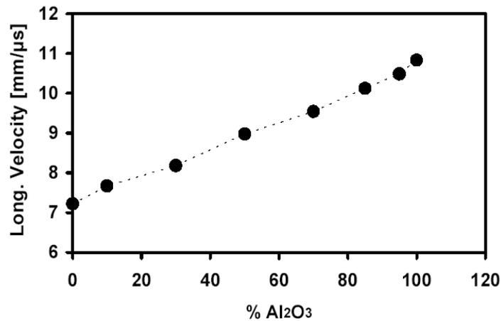
Figure 6.- Longitudinal wave velocity versus the variation of the sintered density of the samples as a function of the % wt Al<sub>2</sub>O<sub>3</sub>.
