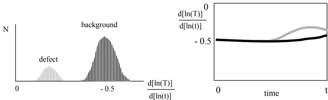
Figure 4: (left) Histogram of logarithmic slope values for a sample with discrete subsurface defect. Background pixels are clustered around a peak value of  $-0.5$ . (right) Time evolution of principal peak values of the logarithmic slope histogram. The secondary (gray) line indicates the emergence of a subsurface defect peak.
