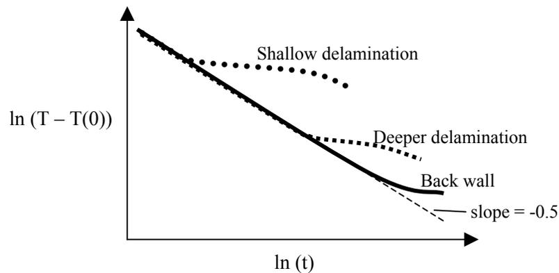
Figure 1: Logarithmic time evolution of the surface temperature. Temperature decay is linear with slope  $-0.5$  until heat flow is obstructed by a subsurface defect or a boundary such as a wall.
