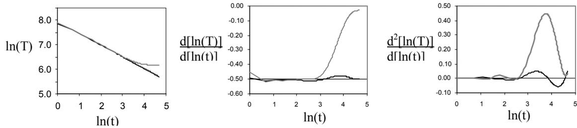
Figure 2: Comparison of logarithmic temperature-time plot of surface temperature of defect and intact points (left) with reconstructed 1<sup>st</sup> and 2<sup>nd</sup> derivatives. Contrast between defect and intact points increases with each derivative.
