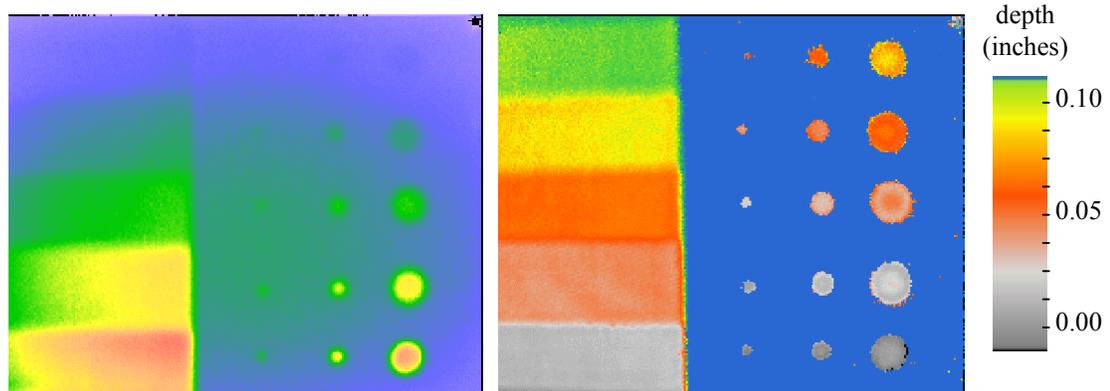
Figure 3. Thermographic images of a composite panel with Rohacell inserts between each ply layers. The inserts in each row are 0.25", 0.5" and 1" in diameter. (left) Raw IR image of the panel 1.6 seconds after flash heating. (right) Depth map created from reconstructed data.
