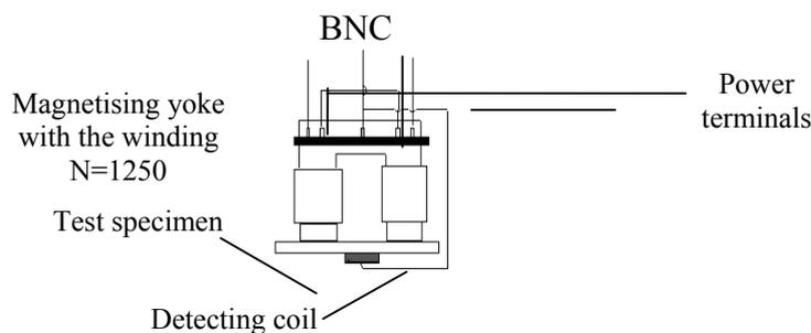
*Fig. 1. Sensor unit with external detection coil.*
