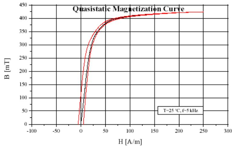
Fig. 4. Magnetisation curve of ferrite material, 12G /12/.
