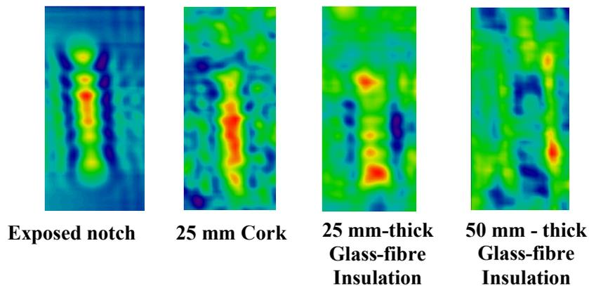
Figure 9. Microwave NDE Images of Surface Breaking Notch Under Insulation
