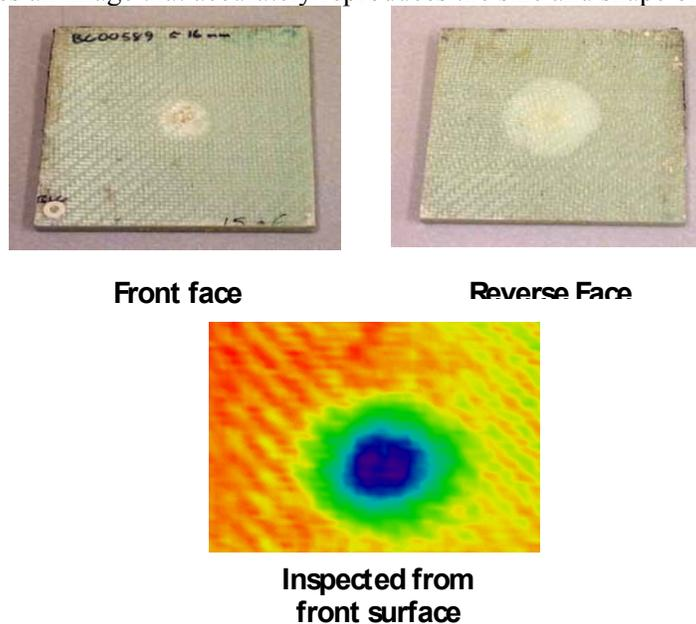
Figure 3. Microwave (35 GHz) Inspection of Impact Damage
