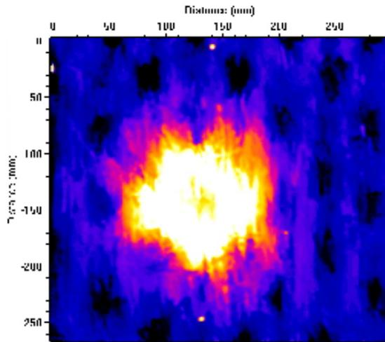
Figure 5. Microwave NDE Image of Core Crushing in a 3.5 mm, e-glass PVC Foam Cored Sample
