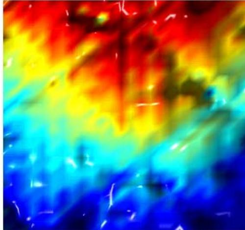
Figure 2. Image of a Triangular Unbonded Outer Skin / Core Joint Inspected from the Inner Skin Side
