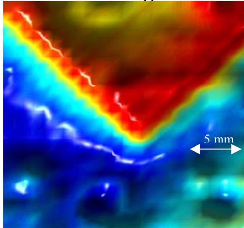
*Figure 1. Image of a Triangular Unbonded Outer Skin / Core Joint Produced at 35 GHz*
