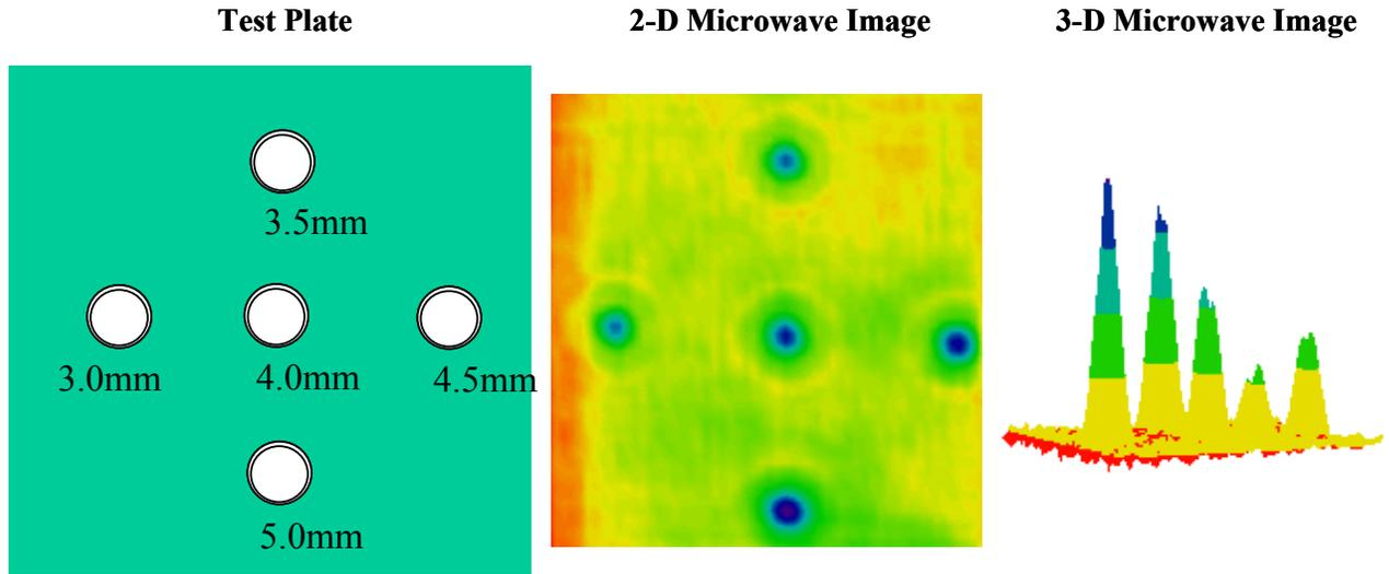
Figure 7. Example of the use of Microwave NDE for the Detection and Measurement of Wall Thinning.
