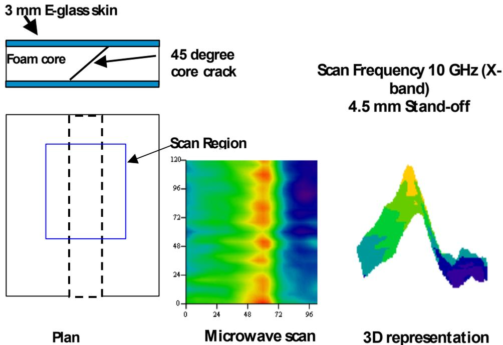
Figure 4. Microwave NDE Image of Core Cracking
