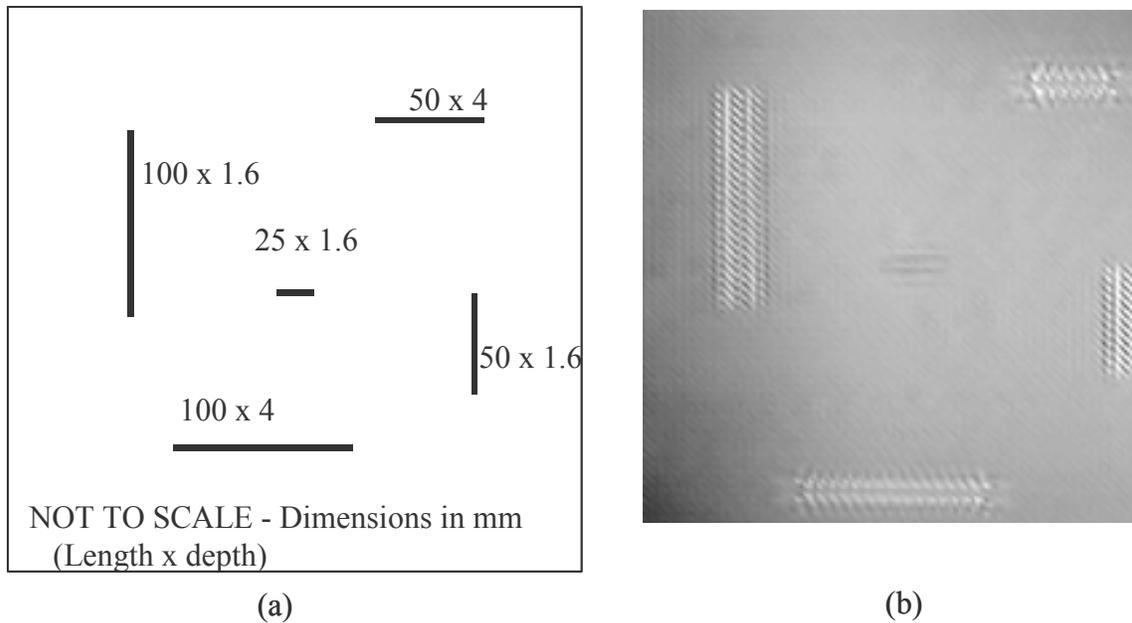
Figure 8. Crack-like Defect Test Plate (a) Dimensions, (b) Microwave Image, Ka-Band
