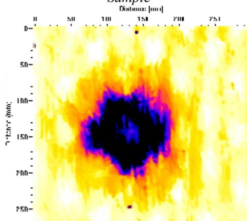
Figure 6. Reverse Palette Image of Core Crushing Defect of Figure 5
