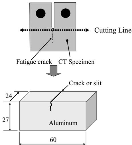
Fig.1 Preparation of cracked specimen
