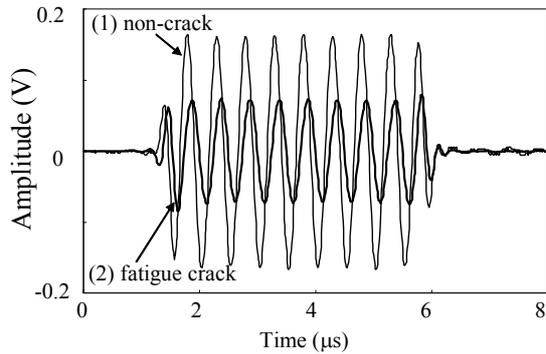
Fig. 8 10-cycle burst waves (2MHz) passing through (1) undamaged and (2) fatigue cracked specimens.
