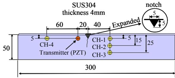
Fig.11 Sensor position for detecting fatigue crack.
