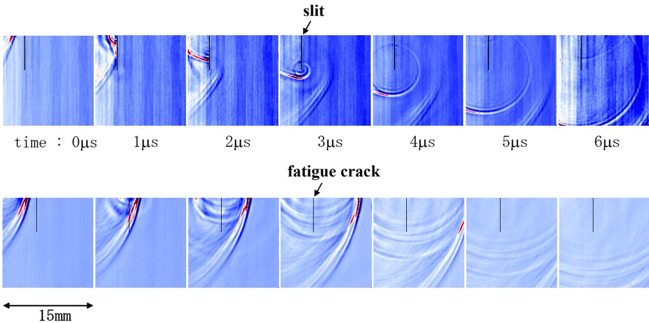
Fig.4 Propagation images of ultrasonics measured around a slit (or fatigue crack). The depth of the slit (or the fatigue crack) is 6mm (or 5.2mm).
