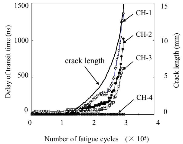
Fig.12 fatigue crack length and delay time of ultrasound at each channel.
