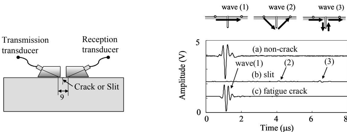
Fig.5 Transducer position for the measurement of burst waves passing through a fatigue crack.
