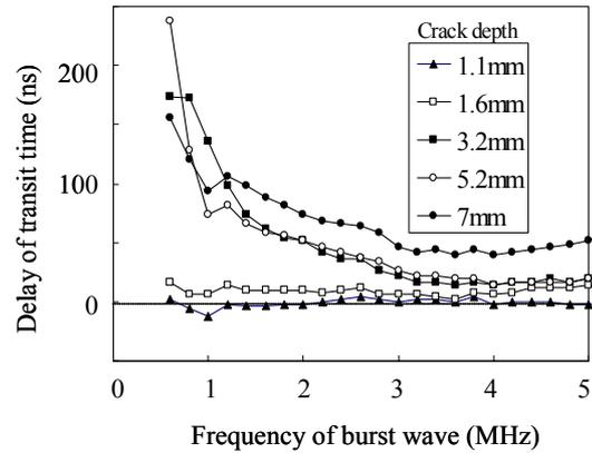
Fig. 9 Effect of burst wave frequency and crack depth on ultrasonic transit times.
