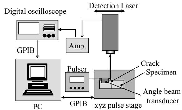
Fig.3 Heterodyne optical system for visualization of ultrasonic waves
