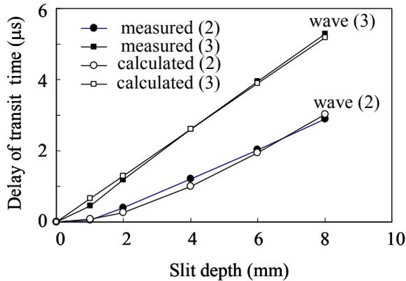
Fig.7 Relationship between slit depth and delay time of ultrasound passing through slits.
