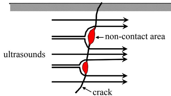
Fig.10 Propagation model of ultrasonics passing through crack interface.
