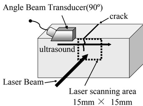
Fig.2 Scanning area of laser beam, and mounting position of an angle beam transducer for visualizing ultrasonic waves.
