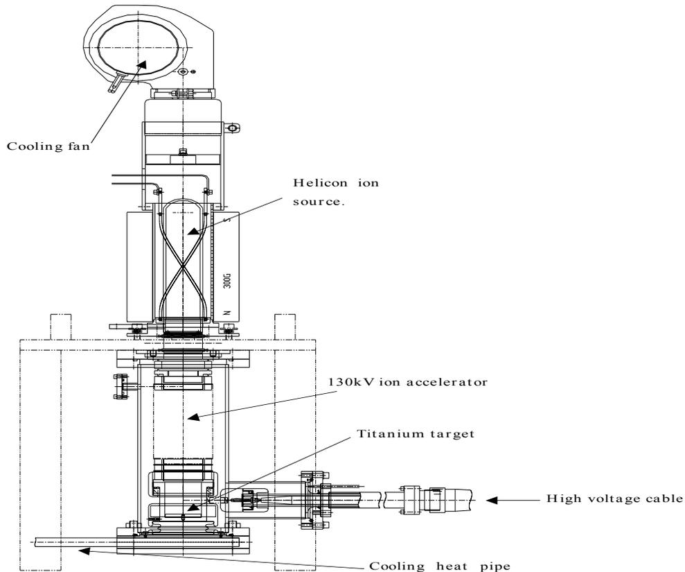
Fig. 1 Schematic view of the neutron generator.
