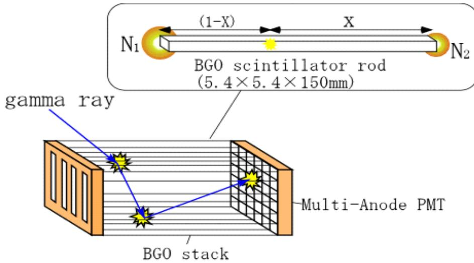
Fig.2 Configuration of a detector unit of multi-Compton gamma camera based on stacked BGO scintillators
