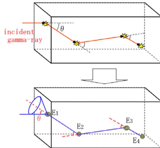
Fig.3 Multiple Compton scattering process
