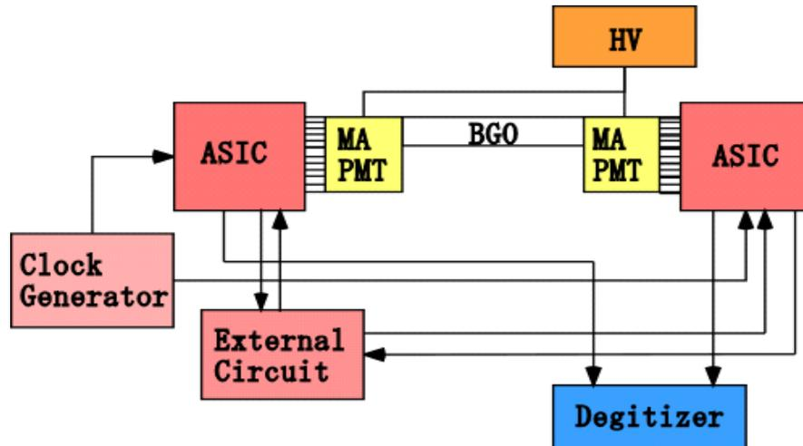
Fig.4 Prototype signal processing system for multi-Compton gamma camera based on stacked BGO scintillators
