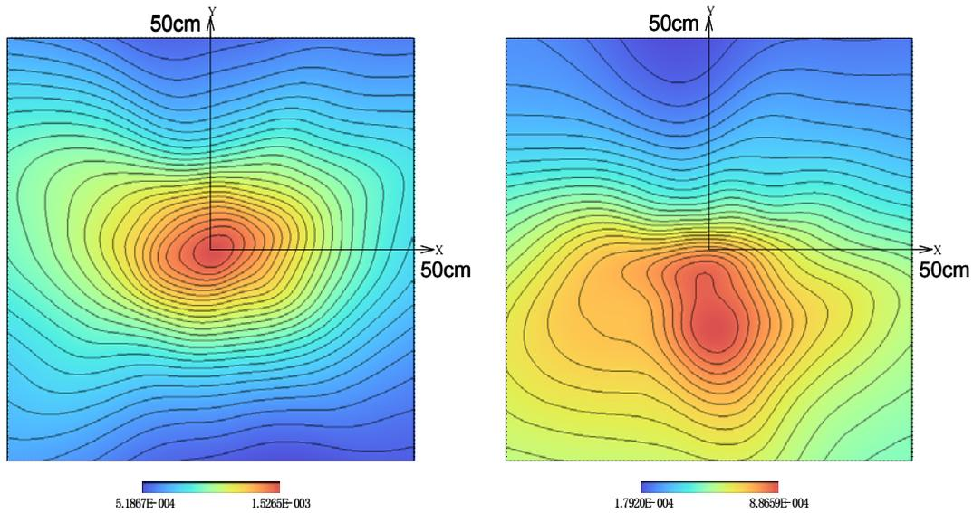
Fig.6 Deduced images for the incident direction of 10.8MeV gamma rays from N of an APM (2cm square x 1cm thick) located at 20 cm depth, and at the center (left) and 20cm apart from the center (right) in a 1m square area, respectively.
