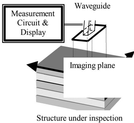
**Figure 1: Near-field waveguide-based imager**
