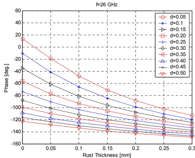
**Figure 3: The phase of the reflection coefficient as a function of the rust thickness and depth as a parameter at 26 GHz**
