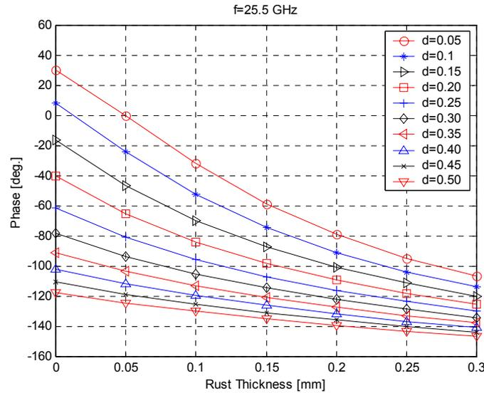
**Figure 2: The phase of the reflection coefficient as a function of the rust thickness and depth as a parameter at 25.5 GHz**
