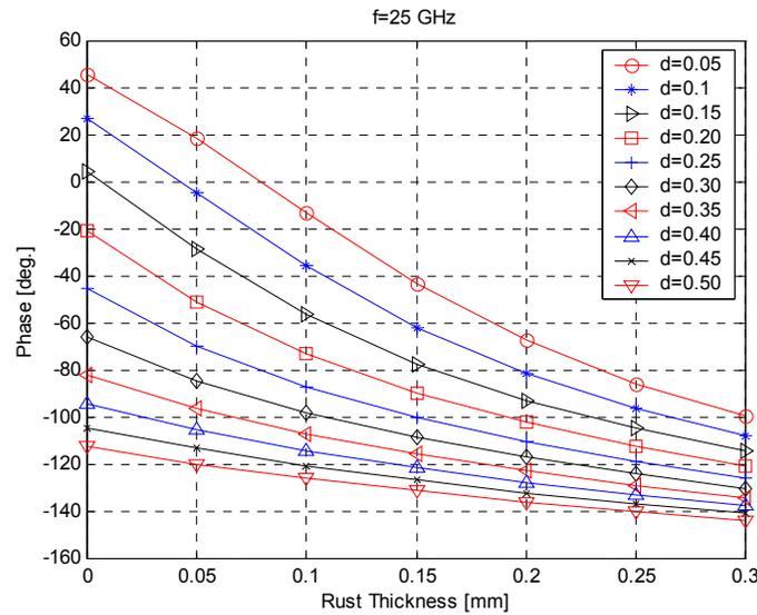
**Figure 1: The phase of the reflection coefficient as a function of the rust thickness and depth as a parameter at 25.5 GHz**
