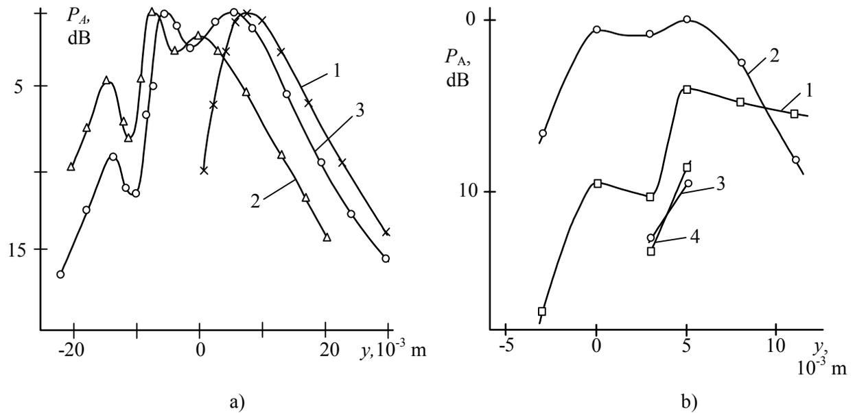
Figure 7. Sound field of STW probe (a) and detection of reference reflectors (b) in steel specimens with having rectangular projection. (a) Waveguide surface is plane (1) and with projection (2, 3); 2 - transverse mode converted from the surface mode; 3- summary field. (b) Waveguide surface with projection (1, 2) and is plane (3, 4);  $l/\lambda=8,4$  (1);  $22,3$  (2);  $0$  (3, 4).
