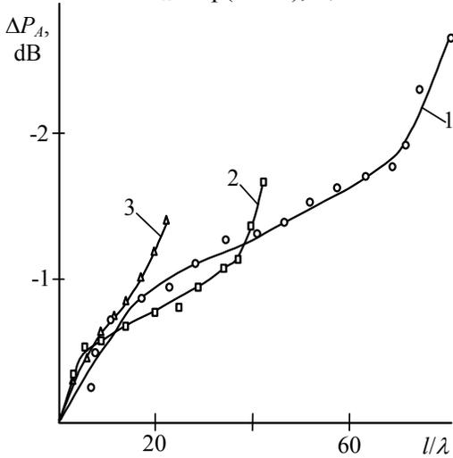
Figure 3. ST (1) and SL (2,3) modes in Aluminum ( $h/\lambda \gg 1$ ).  $L, m=0,15$  (1,2);  $0,08$  (3).
