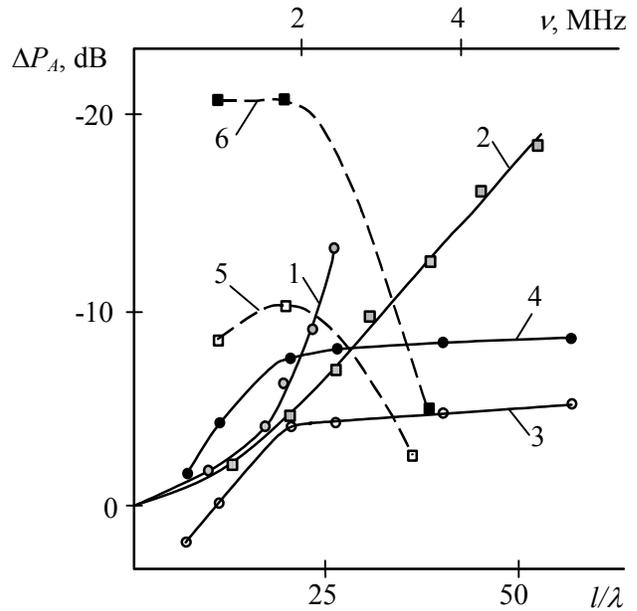
Figure 6. SLW (1, 3, 4) and STW (2,5,6) modes in steel specimen with rectangular projection vs.  $l$  (1, 2) and  $\nu$  (3 - 6).  $L, m=0,035$  (3, 5);  $0,07$  (4, 6).
