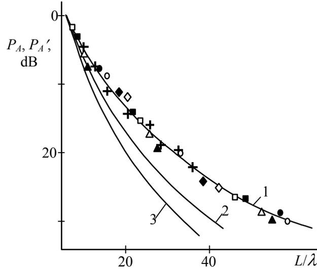
Figure 2. Amplitude of SLW propagating along cylindrical surface vs. distance between probes:  $\varepsilon=0$  (1);  $-0,13$  (2);  $-0,27$  (3, +); probe with cone reflector (+);  $P_A' = P_A \Phi^{-1}(\varepsilon)$ :  $\varepsilon=0,07$  (O, ●);  $0,13$  (? , ?);  $0,22$  (□, ■);  $0,36$  (? , ◆).
