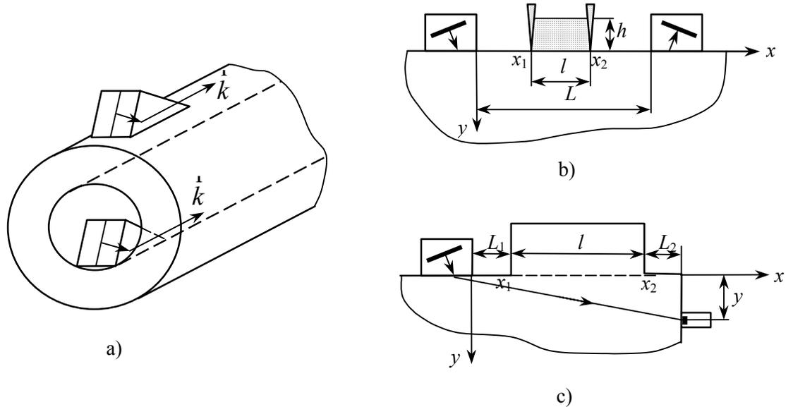
Figure 1. Schematic diagram of ultrasound generation and receiving.
