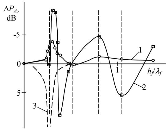
Figure 4. Amplitude oscillation in pulse of SLW (1, 2) and surface mode (3) [5] vs. fluid height  $h_f$ . Number of oscillation in pulse: 2 (1); 5 (2).
