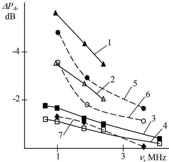
Figure 5. Pulse amplitude of SLW (1-4) and STW (5-7) vs. frequency when fluid layer put on waveguide surface. Solid: Plexiglas (1, 2); Aluminium (3-6); steel (7).
