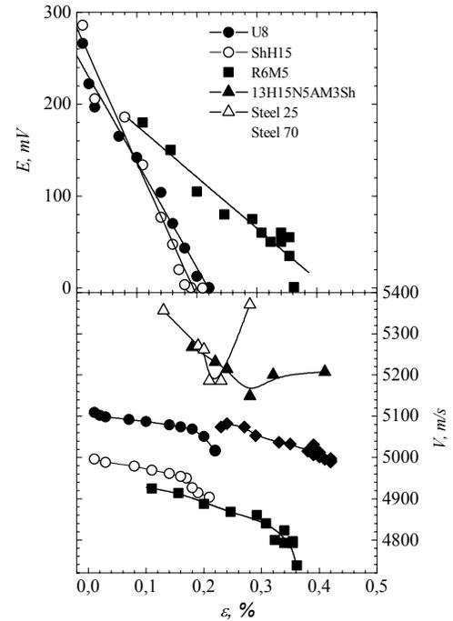
Fig.2. EMAT amplitude  $E$  and elastic wave velocity  $V$  as dependent on microdistortions  $\varepsilon$  for steels 25, 70, U8, ShH15, R6M5, 13H15N5AM3Sh.
