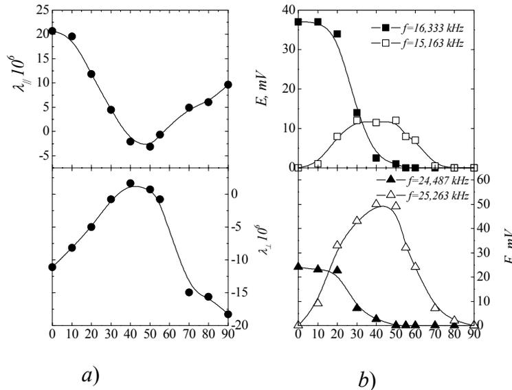
Fig.4. Longitudinal  $\lambda_{\parallel}$  and lateral  $\lambda_{\perp}$  magnetostriction corresponding to the maximum EMAT signal amplitude (a) and EMAT signal amplitude for different resonant frequencies (b) as dependent on the angle  $\alpha$  between the easy direction of magnetization [001] of a monocrystalline Fe-3%Si disk and the direction of the polarization magnetic field  $H_{opt}$ .
