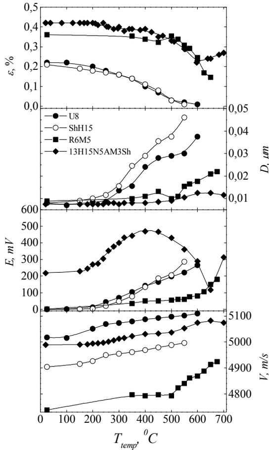
Fig.1. Microdistortions  $\varepsilon$ , typical dimension of coherent scattering regions  $D$ , EMAT amplitude  $E$  and elastic wave velocity  $V$  as dependent on tempering temperature  $T_{temp}$  for steels U8, ShH15, R6M5, 13H15N5AM3Sh.
