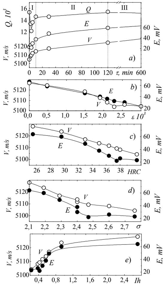
Fig.3. EMAT amplitude  $E$ , elastic wave velocity  $V$  and the EMAT signal quality factor  $Q$  as dependent on the duration of annealing  $\tau$  at  $650^\circ\text{C}$  (a); EMAT signal amplitude  $E$  and sound velocity  $V$  as dependent on microdistortions  $\varepsilon$  (b), hardness HRC (c) and wear resistance  $\sigma$  (d), wear rate  $I_h$  (e) for steel U9.
