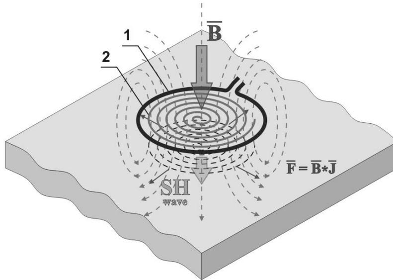
**Figure 1. The scheme of EMA sending-reception of SH-waves with radial polarization with pulse magnetic biasing**
