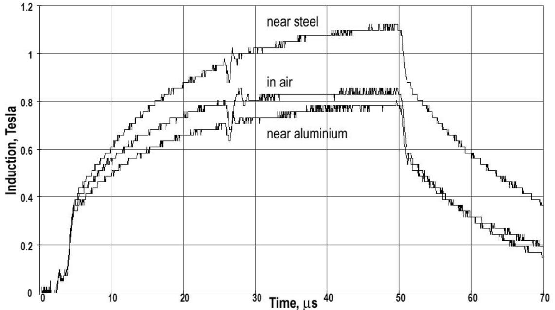
**Figure 2. Dependence of magnetic field induction on time near the operation surface of EMAT**
