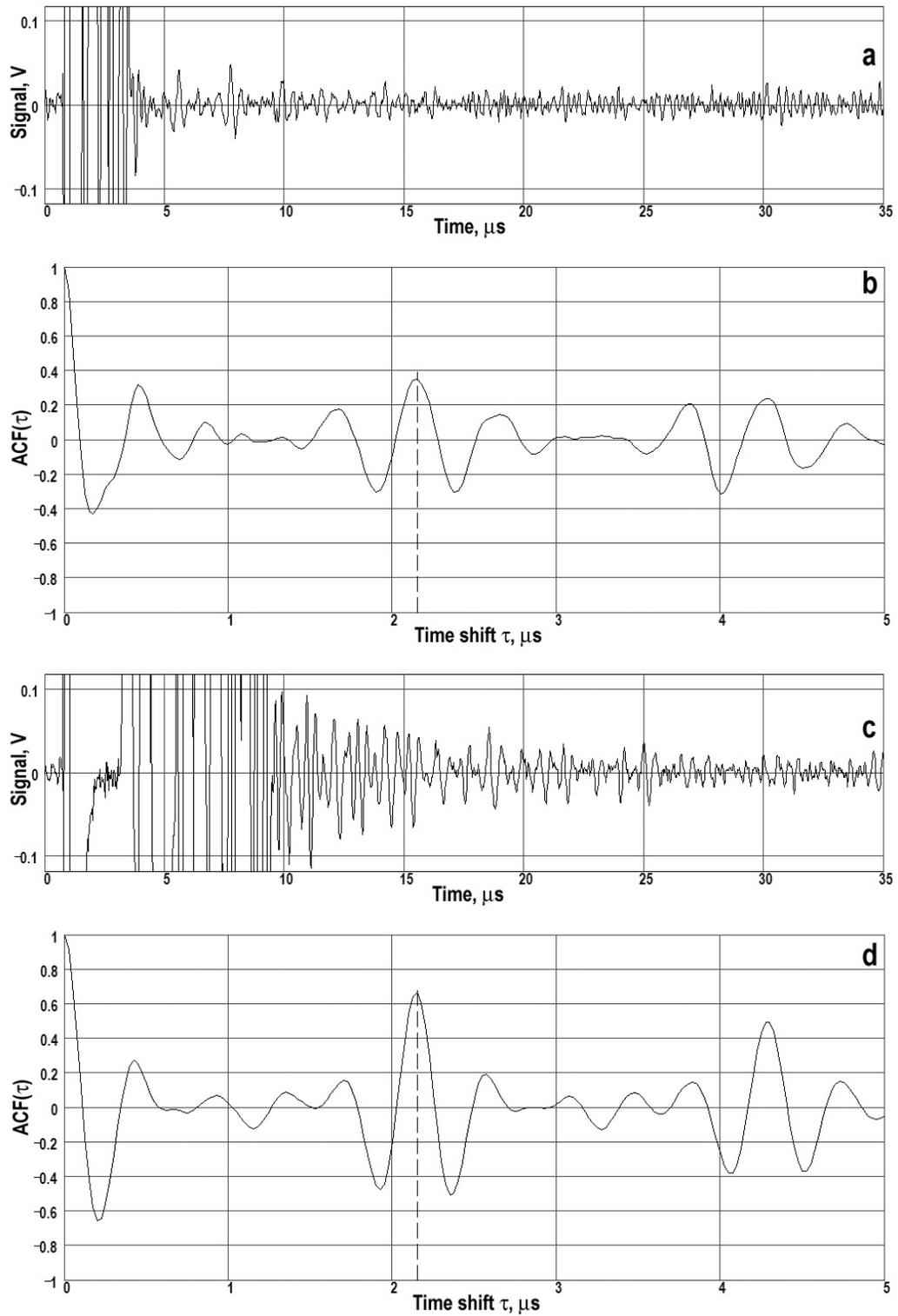
**Figure 5. Realizations of received signals and ACF for EMAT excitation of SH-wave in a steel tube with corroded surface with:**
