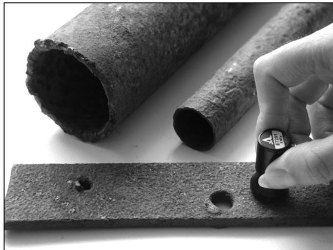
**Figure 6.** The process of corroded steel rolling samples testing by EMAT with pulse biasing
