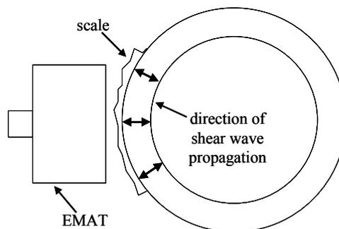
Figure 6 – direction of wave propagation
