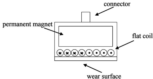
**Figure 2 – cross section of typical EMAT**
