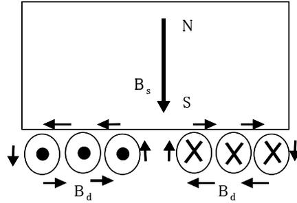
Figure 3 – method of sound wave generation
