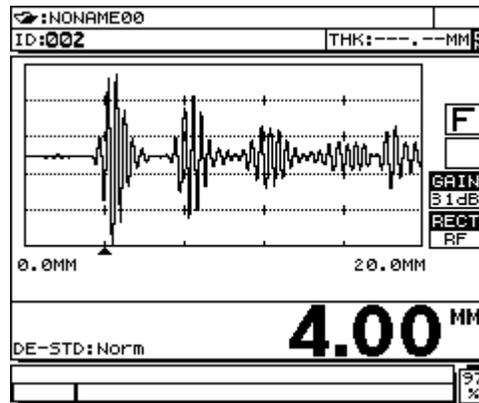
Figure 5 – typical piezoceramic transducer waveform
