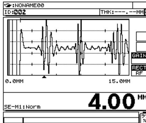
Figure 4 – typical EMAT waveform
