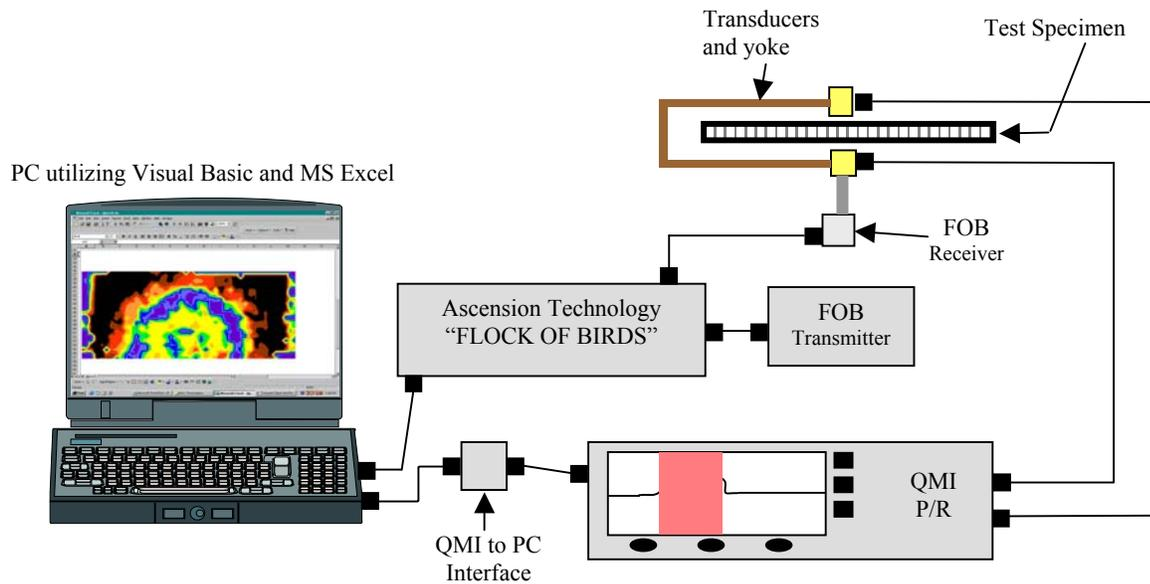
Fig. 6 Schematic diagram of the manual air-coupled ultrasonic scanning system
