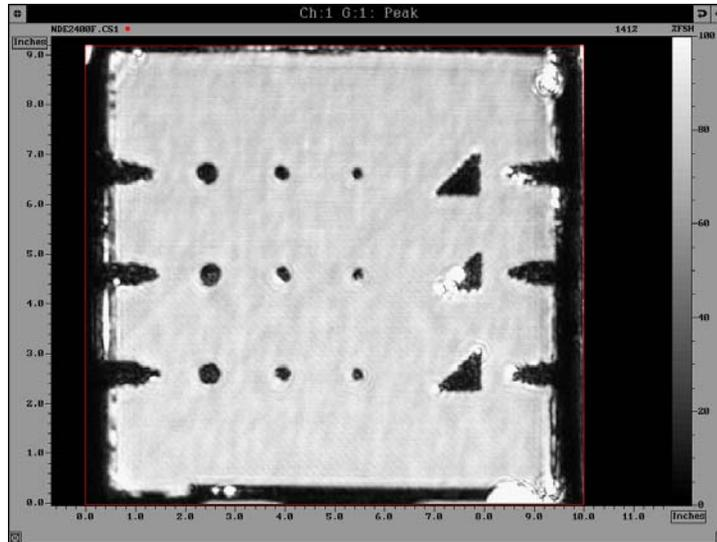
Fig. 3 Air-coupled transmission ultrasonic image of flaws in a 10-ply CFRP.
