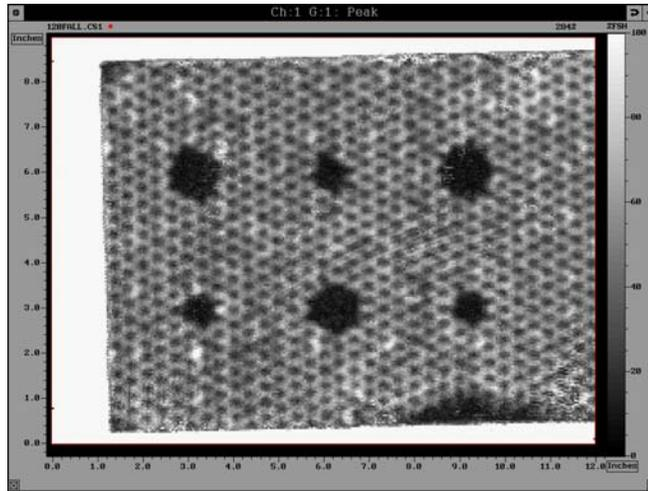
Fig. 4 Disbonds in aluminum honeycomb sandwich revealed by AC-UT transmission C-scan.
