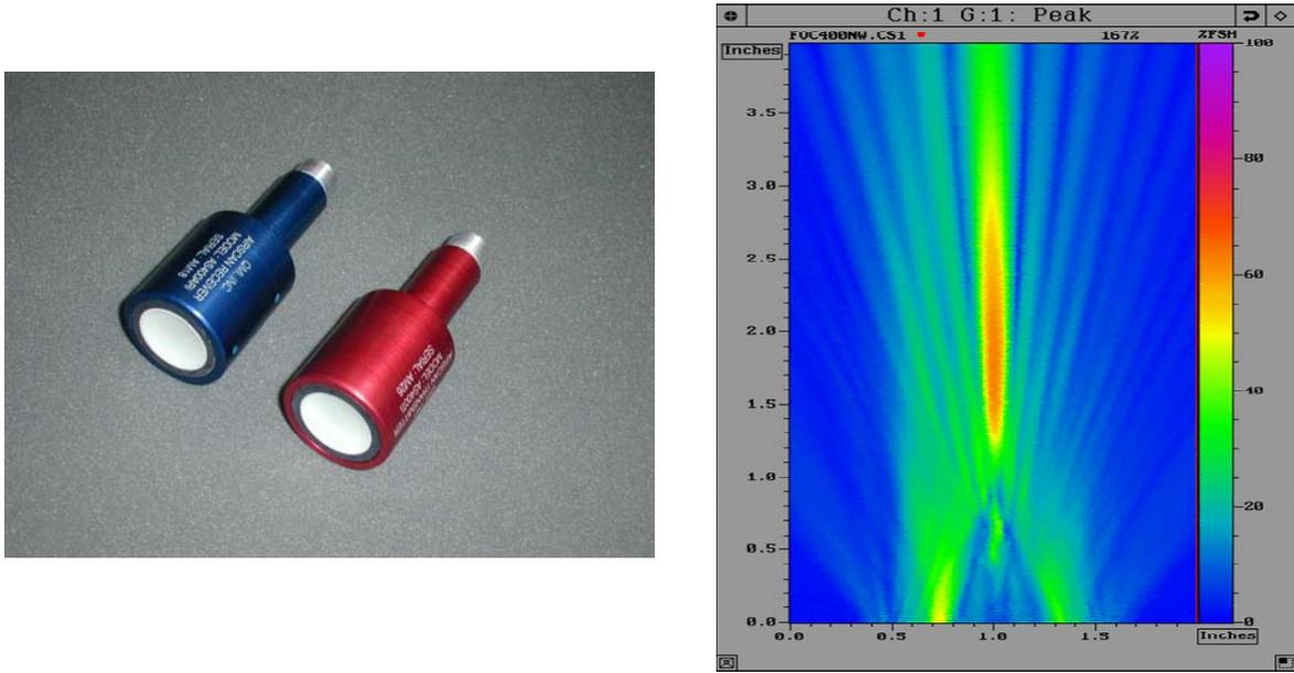
Fig. 1 Piezoceramic air-coupled transducers and field profile of a focused probe.
