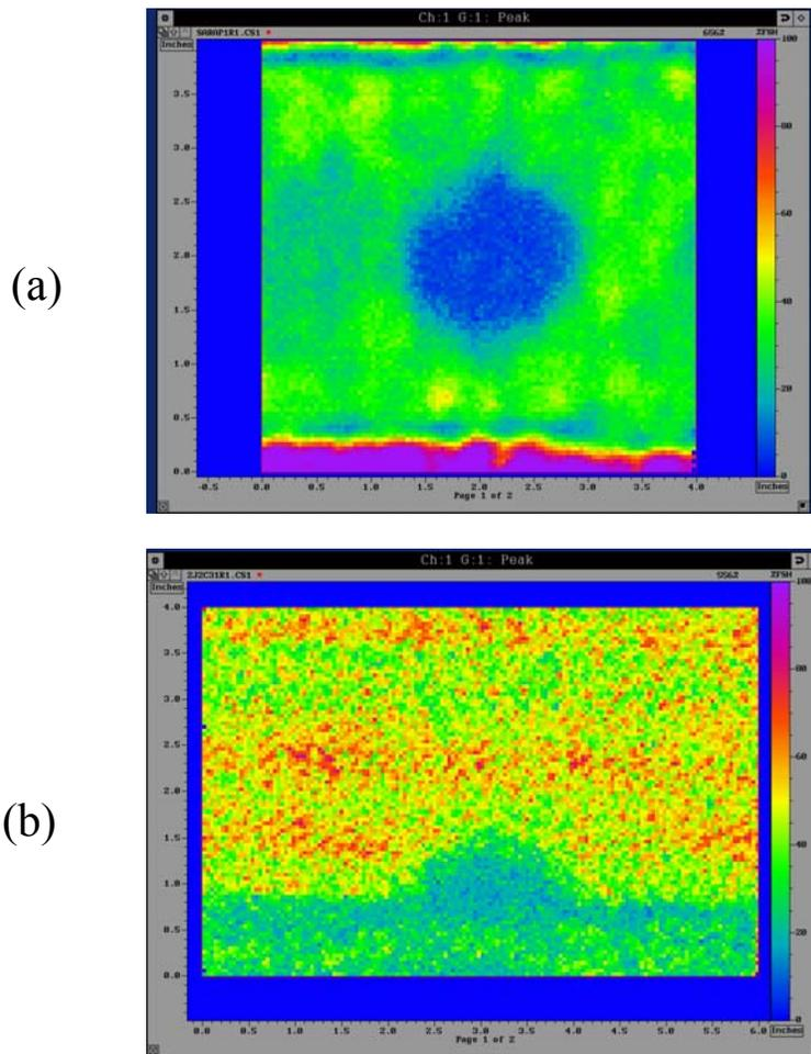
Fig. 5 Air-coupled ultrasonic transmission C-scan of a visible impact damage (a) and one-half of a nonvisible impact damage (b).
