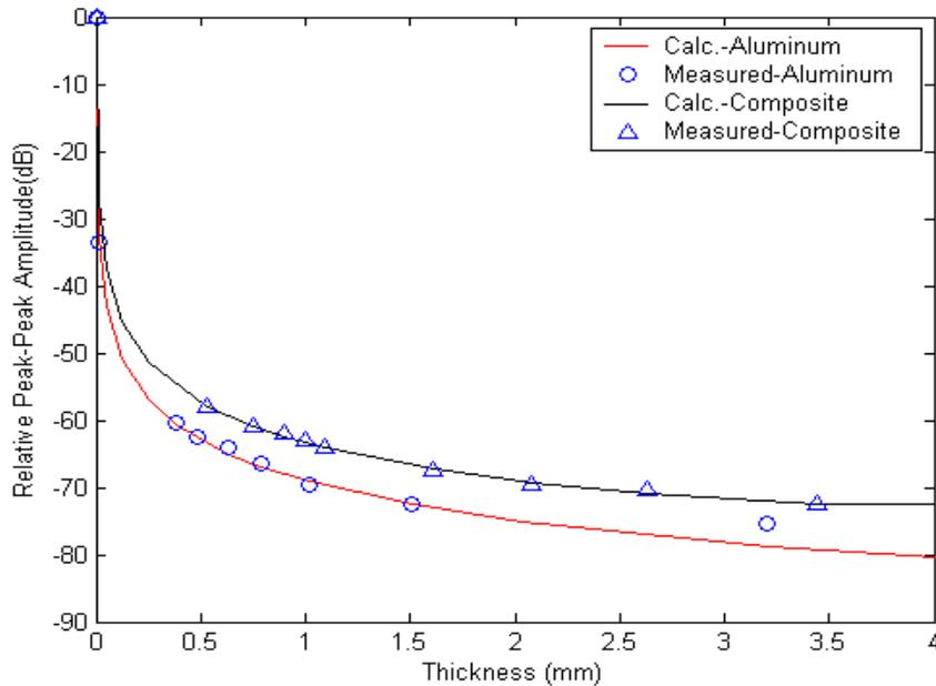
Fig. 2 Comparison of measured and calculated signal transmission of a 120 kHz toneburst.
