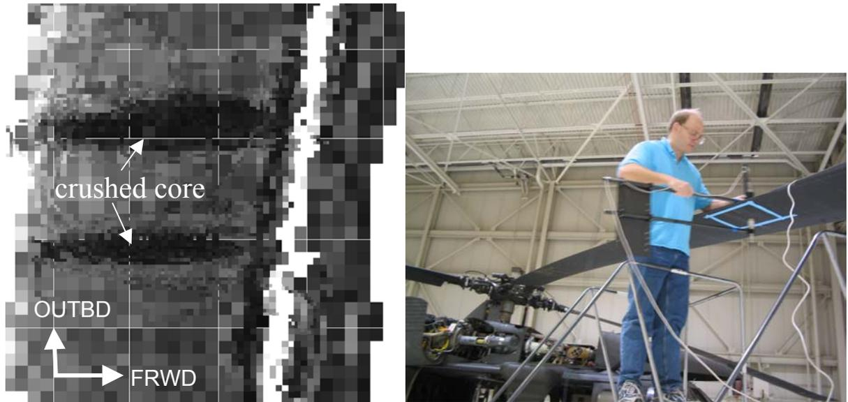
Fig. 8 Damages of a helicopter rotorblade as imaged by the manual AC-UT scanner.
