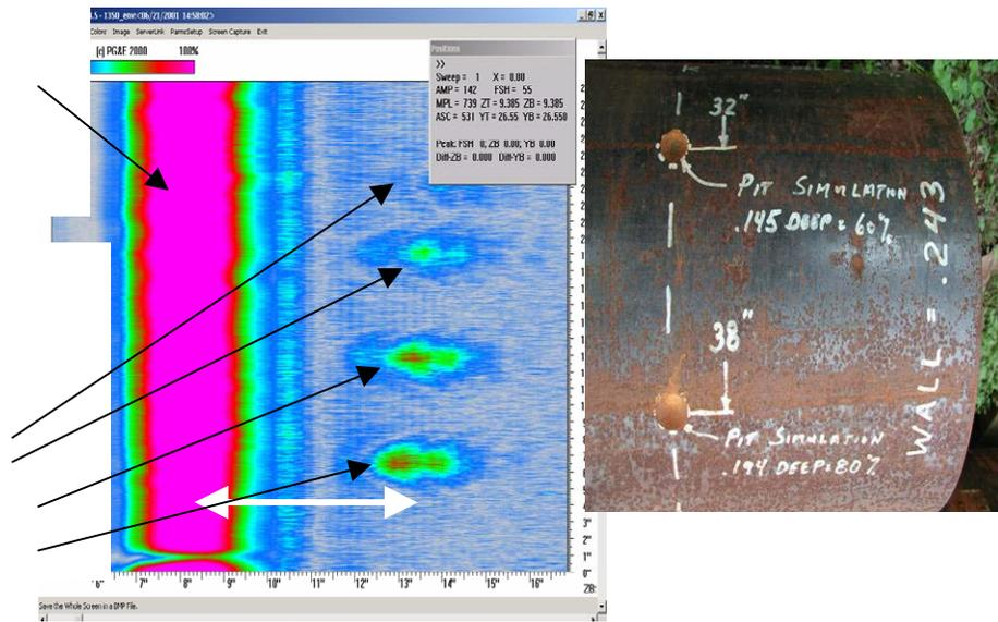
Figure 2. Example of an **E-scan** of a 14” diameter x 0.25” wall pipe containing simulated corrosion pits in the form of 1” diameter, hemispherical depressions with depths of 0.050” (20%), 0.102” (40%), 0.145” (60%) and 0.194” (80 %).
