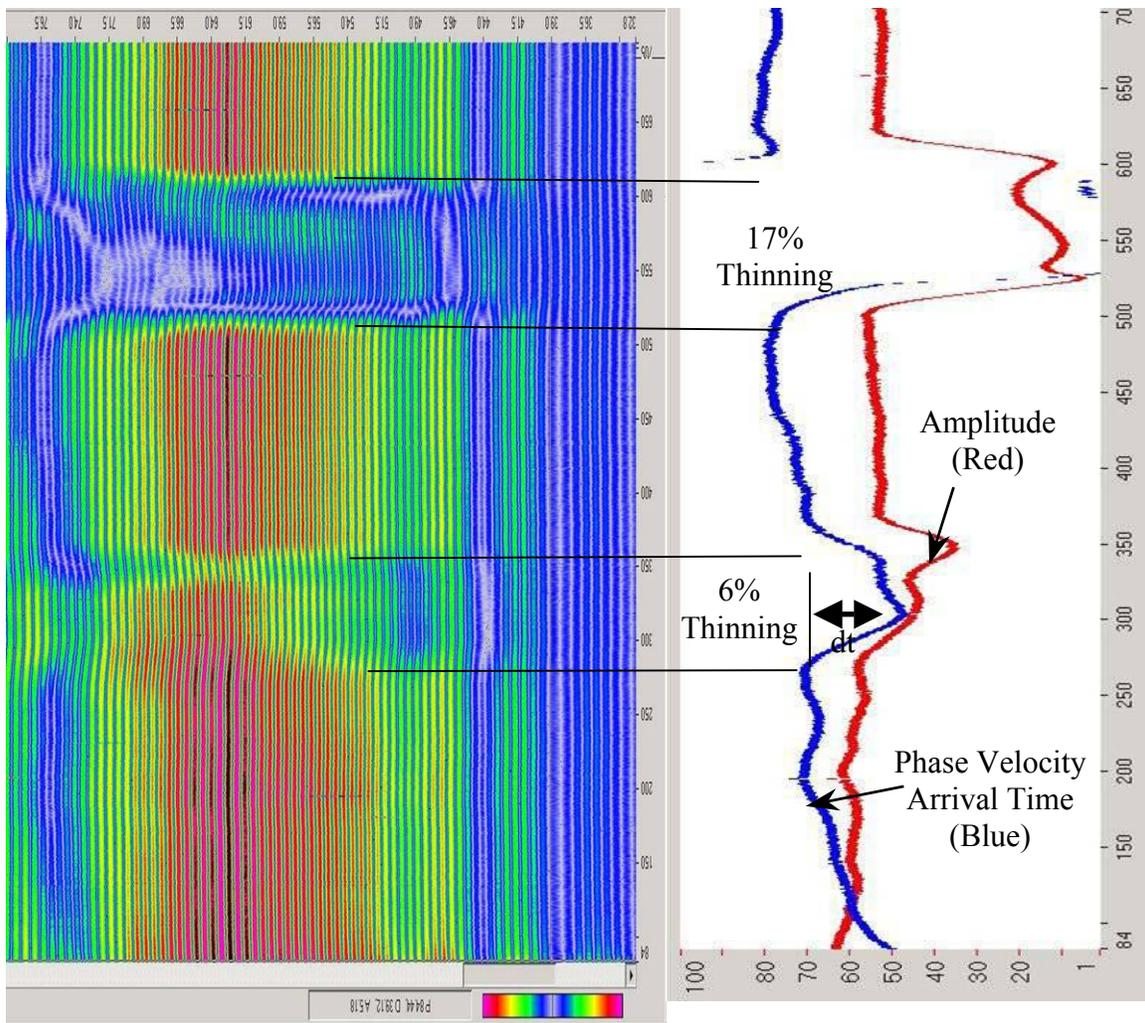
Figure 4. Line Graph Enhanced display of an E-scan. (Left) E-Scan of Lamb wave through two localized thin areas. The change in amplitude was clear but the change in arrival time through the 6% thinning was less obvious. (Right) Line graphs of the amplitude and phase velocity enhance the change in velocity through the 6% thin area.
