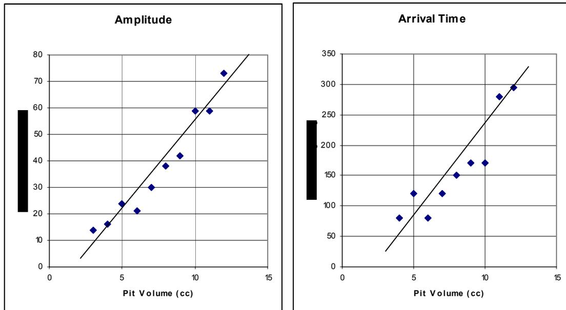
Figure 5. Correlation observed between the amplitude drop and the shift in transit-time of a guided wave passing through real corrosion and the volume of that corrosion.
