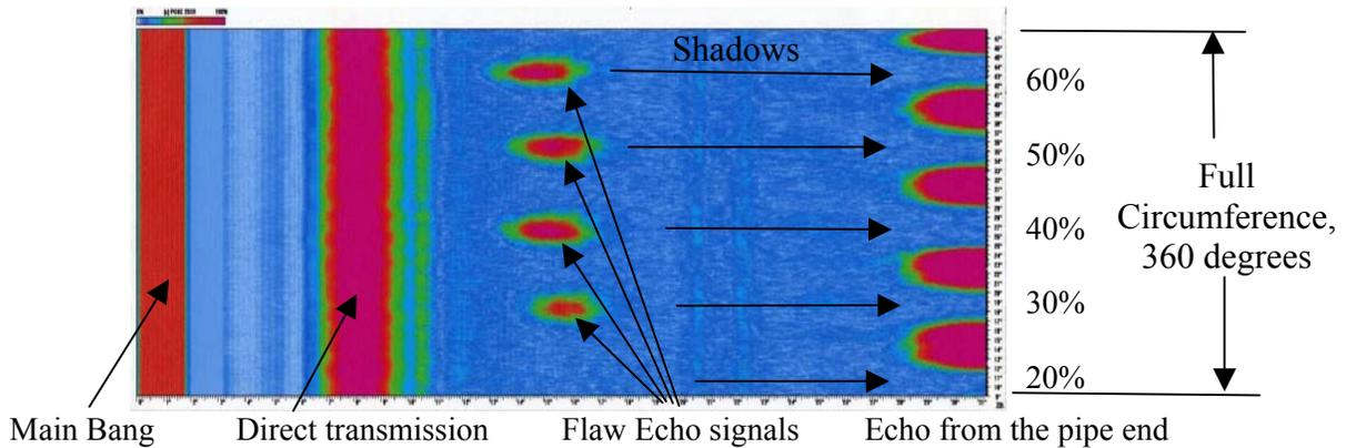
Figure 3. Complete E-scan of five simulated hemispherical thin areas in a pipe. The horizontal or time-of-arrival axis has been expanded to show the “Main Bang” at time=zero, the Direct Transmission signal at a time determined by the transmitter-receiver separation distance, the flaw echo signals whose times-of-arrival are determined by the distance between the EMATs, and the shadow of the flaw cast in the echo from the end of the pipe.
