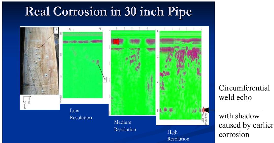
Figure 6. Three E-scan presentations of a field of general corrosion and pits near a circumferential weld in a 30" diameter pipe.
