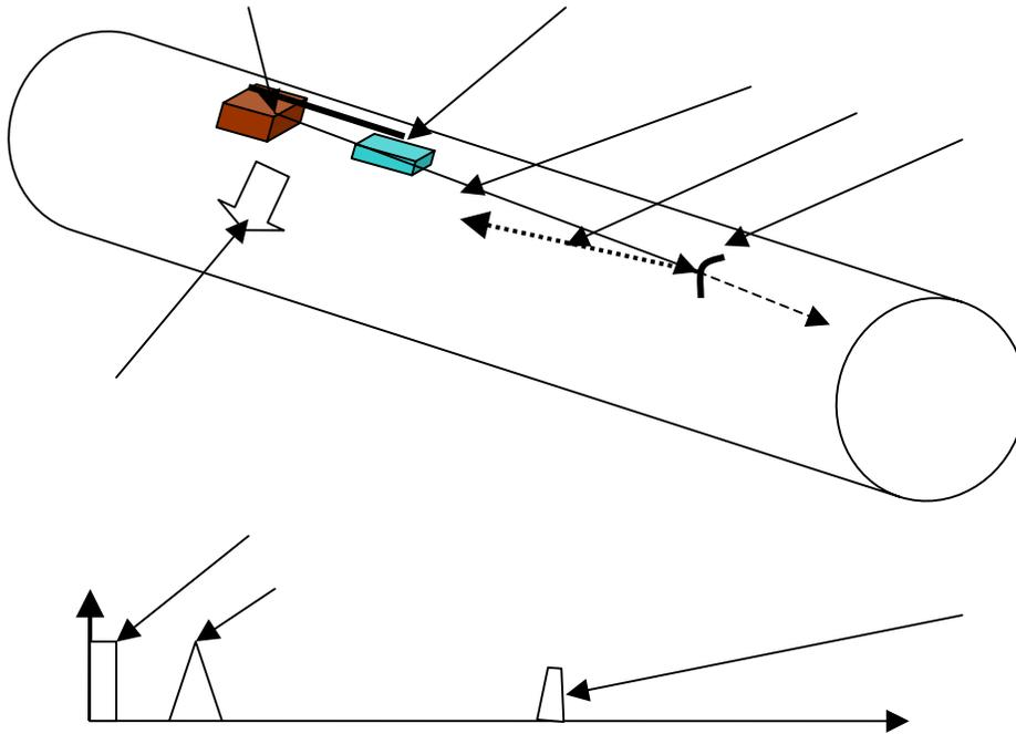
Figure 1. Schematic diagram of an EMAT system for inspecting a cylinder or pipe using guided waves propagating in an axial direction.
