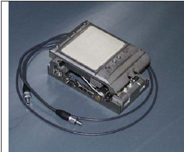
Fig. 12: SH-wave probe
