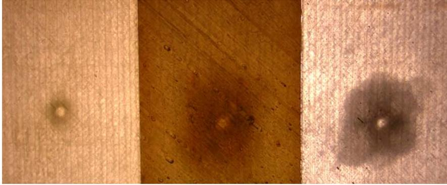
Figure 3 Colour change and loss of transparency of plates. The left most has been in water at 65° C for one week, the middle one has been in water for one week at 93° C and the right hand most has not been exposed to water.
