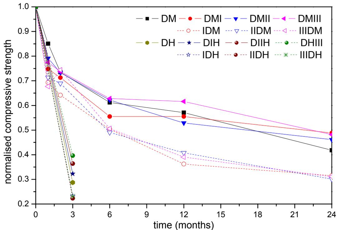
Figure 8 Normalized compressive strength for specimens immersed in water at 65° C marked M and 93° C marked H, with respect to time. Specimens with dashed lines correspond to results obtained for specimens impacted after water immersion. The roman numerals I, II and III relate to the impact level 2.5, 5 and 10 Joules, when before the specimen name correspond to impact after water immersion.
