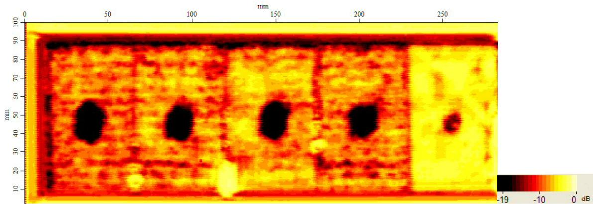
Figure 5 A series of specimens scanned after 24 months in water at 65° C. The last specimen on the right has not been exposed to water. The four specimens in the left have been impacted with 5 J prior to immersion in water. The unexposed specimen has been impacted at 2.5 J. Scan step size 0.8 mm, scan speed 25 mm/sec. The very bright spot between the four specimens on the center is due to some gap between the specimens allowing direct transmission to the receiver probe.
