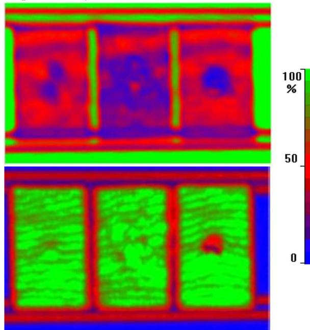
Figure 4 A series of specimens type D that have been impacted at 10 J. The first row depicts amplitude measurement with the gate at the bottom of the specimen. The bottom row has the gate set near the surface of the samples. The left most was impacted and exposed at 65C for 2 months. The middle has been impacted but not
