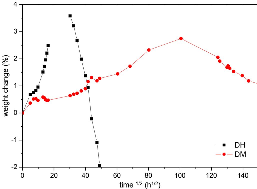
Figure 1 Water uptake results for specimens held at 65° C marked DM and at 93° C marked as DH.
