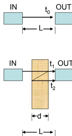
Figure 6 The acoustic wave velocity measurement set up.
