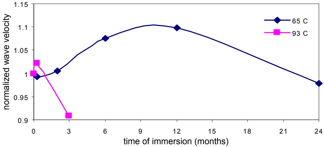
Figure 7 Normalized wave velocity through the material with respect to time of immersion. Normalization is against the dry sample, at time 0.
