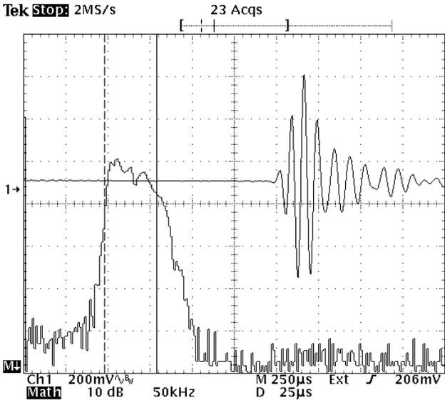
Fig. 4. 100 kHz, 50x50 mm. Sensitivity: -46 dB.
