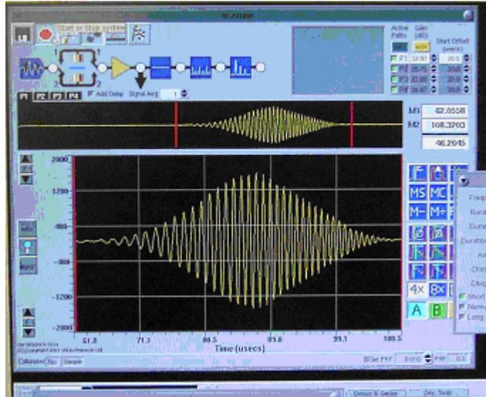
**Figure 4- Chirp signal**
