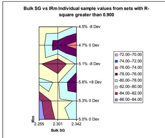
Figure 12- Contour plot of individual sample values from sets with R-square greater than 0.900
