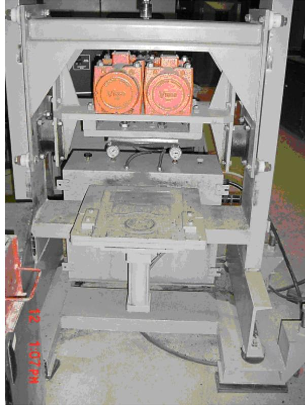
**Figure 3- Vibratory beam compactor**
