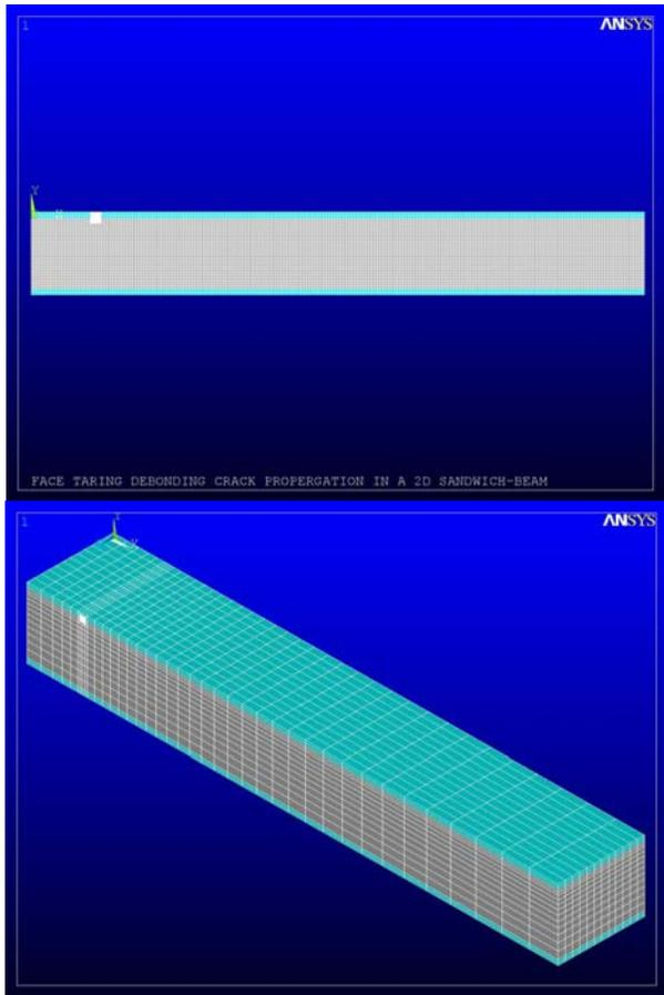
Figure 5. Finite element models used for crack length prediction. The 2D model (left) and the 3D model (right)
