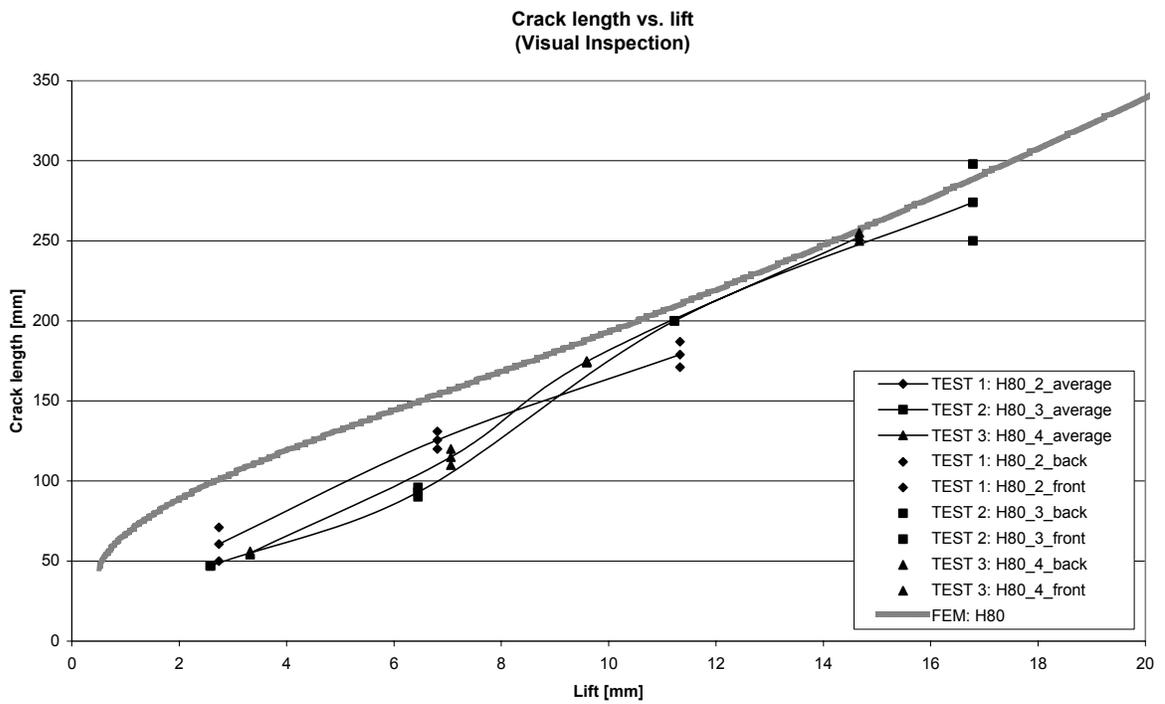
Figure 7. Correlation between the lift of the skin layer and crack length based on visual inspection.
