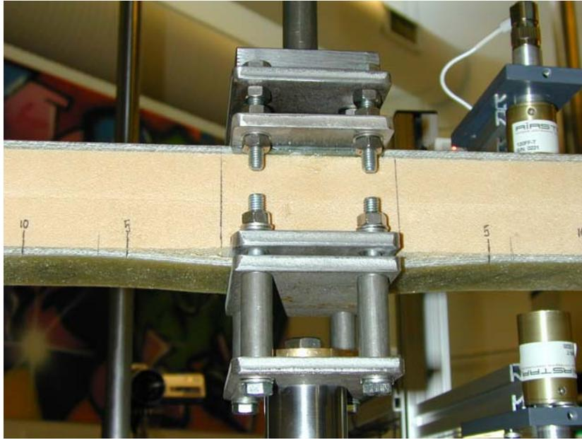
Figure 2. In-situ ultrasonic scanning system. To the right the two air-coupled transducers in through-transmission set-up are seen. The distance to the specimens is 15 millimetres
