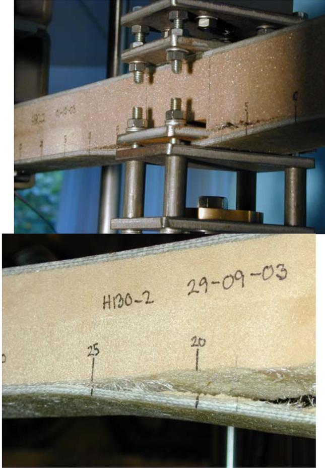
Figure 3. Sub-interface crack propagation in H80 specimen (left) and interface propagation with fibre bridging in H130 specimen (right)
