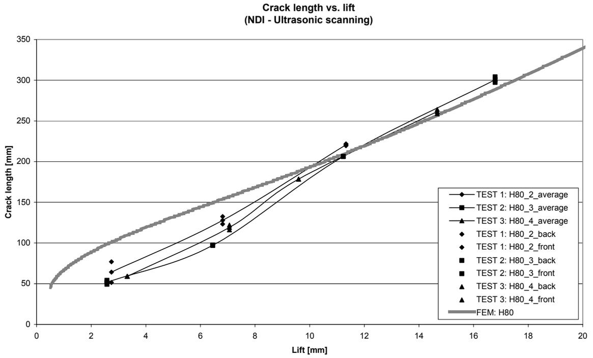
Figure 6. Correlation between the lift of the skin layer and crack length based on ultrasonic results.
