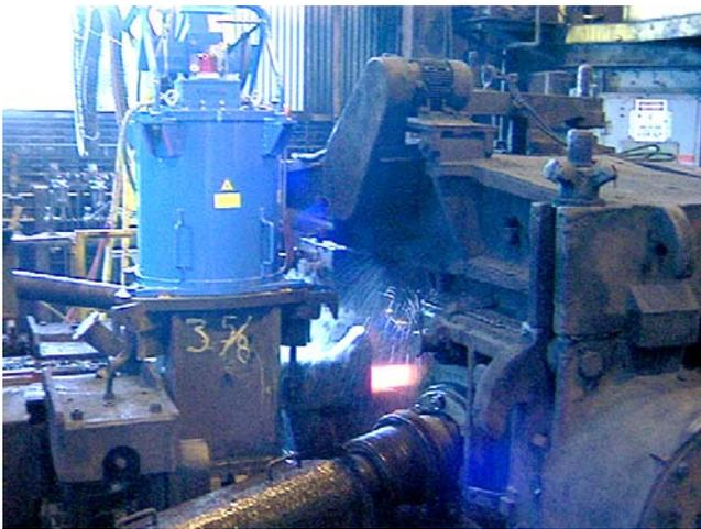
Figure 7. View of the inspection head located on-line measuring a tube being processed.
