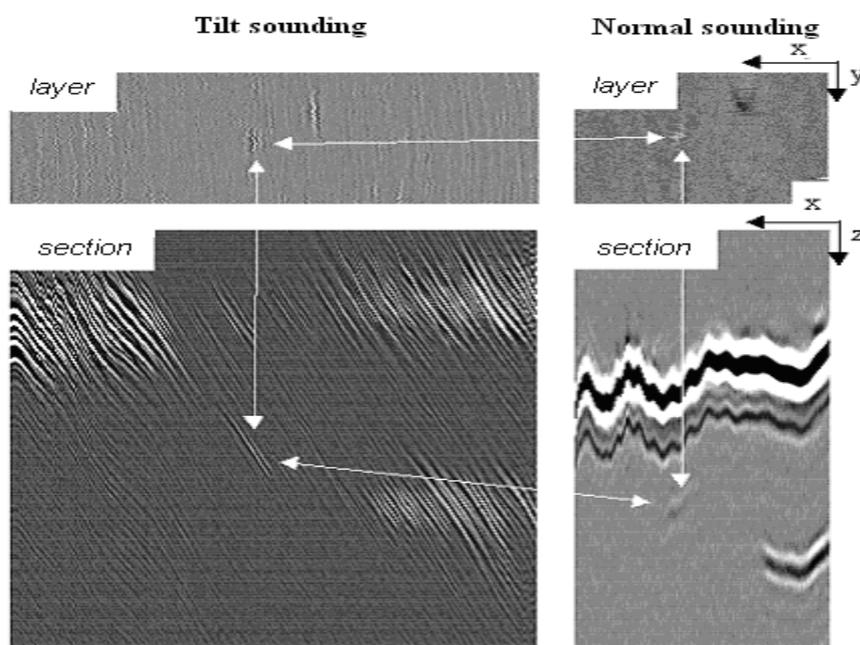
**Fig.2.** Layer and section images according to inclined and normal sounding
