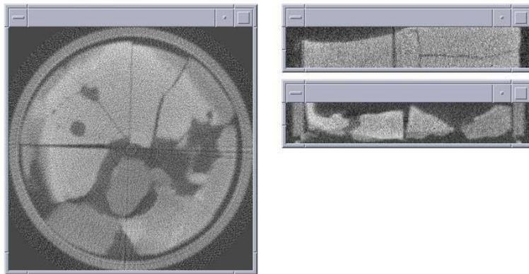
Figure 5: Slices of the cone-beam reconstructed volume, concrete test block.
