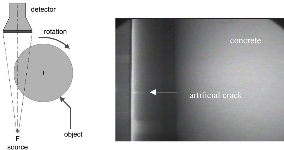
Figure 4: Tangential tomosynthesis, geometry (left) and example of tomosynthesis result (right).
