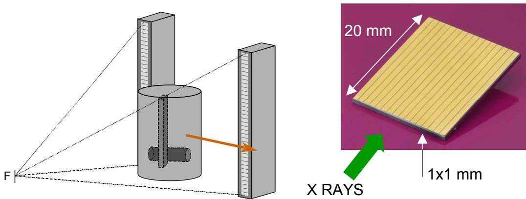
Figure 3: Radiography by translation, geometry using 2 arrays (left) and CdZnTe array (right).
