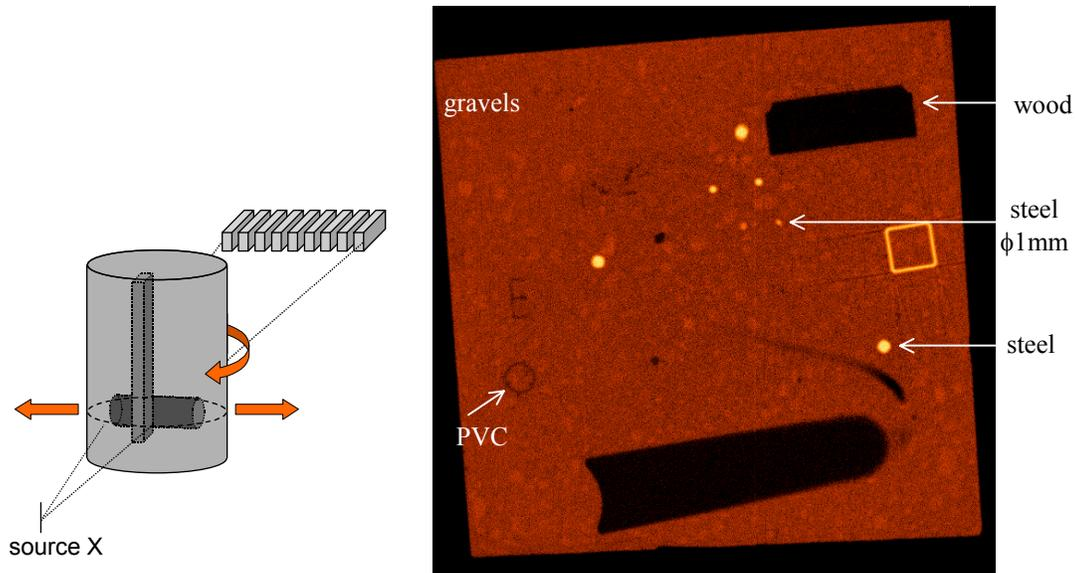
Figure 6: Tomography using translation-rotation, geometry (left) and result (right).
