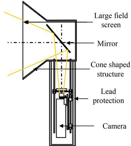
Figure 1: *left*: example of waste drum in concrete package (weight 1210 kg, diameter 840 mm), *right*: diagram of the large field detection system.
