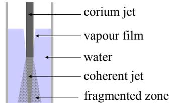
Figure 1: diagram of experiment principle
