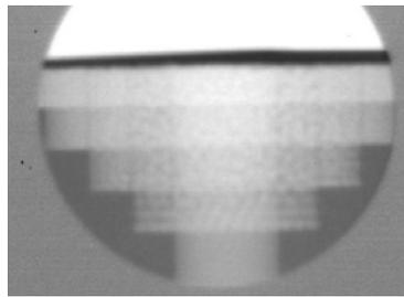
Figure 6: image of a steel bar ( $\varnothing$  30 mm) sunk in steel balls
