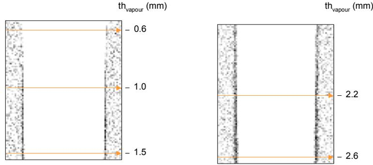
Figure 3: image simulated by Sindbad: source 6 MeV 0.3 Gy/s, 10 ms integration
