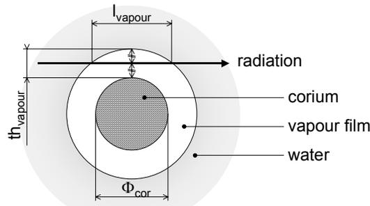
Figure 2: geometry of the vapour film around the coherent corium jet
