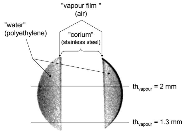
Figure 4: experimental image: vapour film around a corium jet (simulated by stainless steel); the altitudes marked on the image indicate film thickness  $th_{\text{vapour}}$ ; integration 17 ms; source 8 MeV, 0.06 Gy/s
