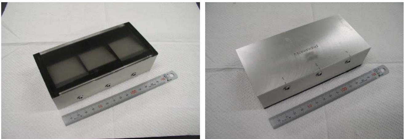
Fig.6 A view of the newly made surface SH transducer with three elements
