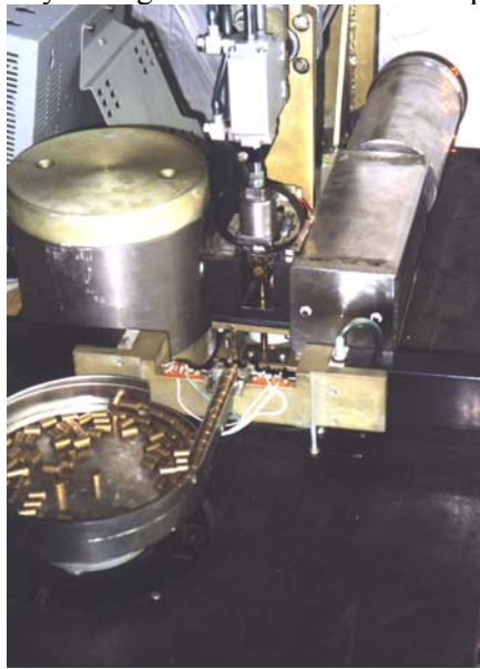
Fig. 1. The device for diameter and density testing of sintered fuel pellets.
