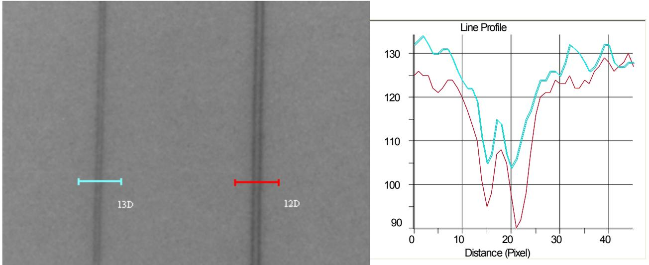
**Fig. 4 Resolution measured according to EN 462-5 (400 kV, 20 mm steel)**
