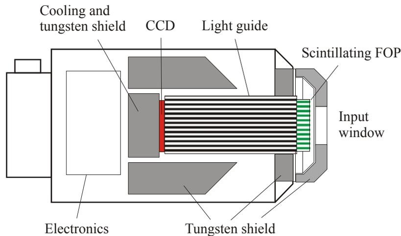
**Fig. 3 Schematic sketch of the x-ray imaging detector.**
