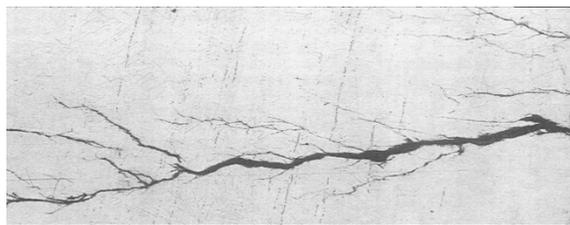
**Fig. 1** Cross section of an typical IGSCC.
