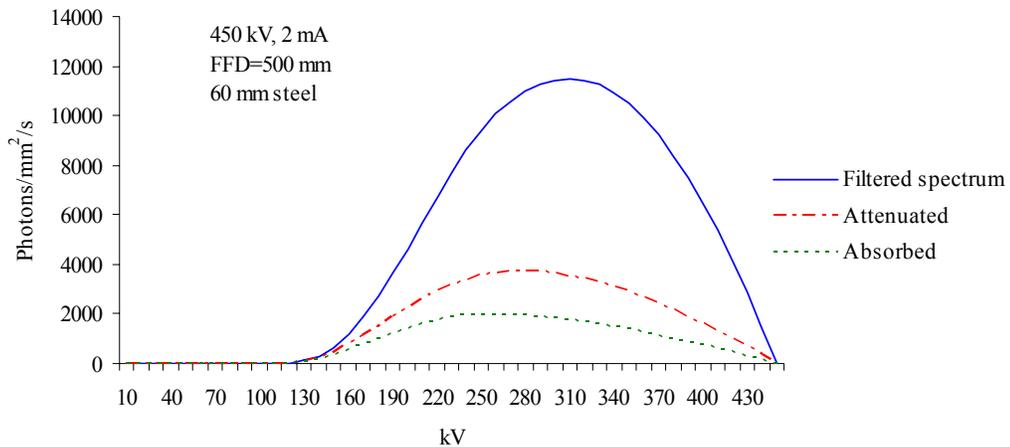
**Fig. 2 Simulated filtered spectrum and detection efficiency of a 10 mm scintillating FOP.**
